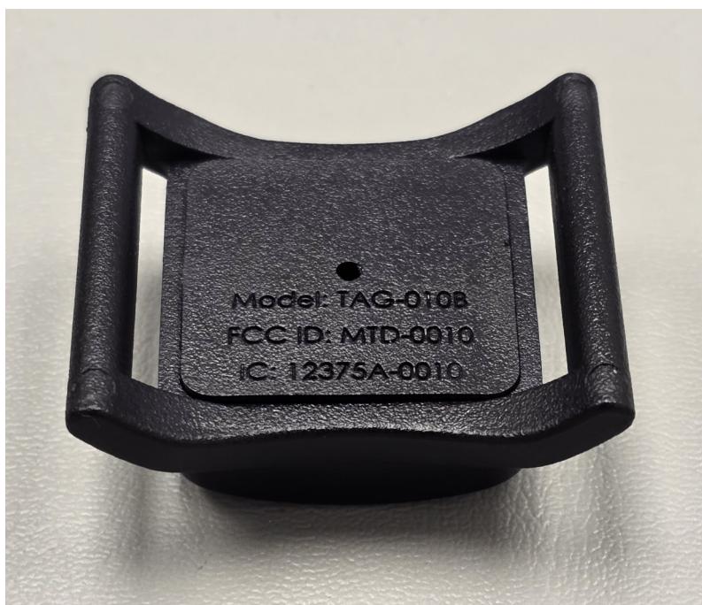
Assembled unit with potting and Cover
