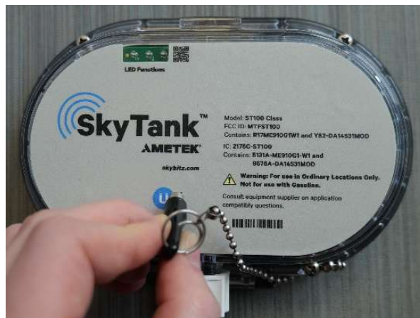
Figure 2: ST100 Gateway unit being magnet swiped over blue magnet indicator
