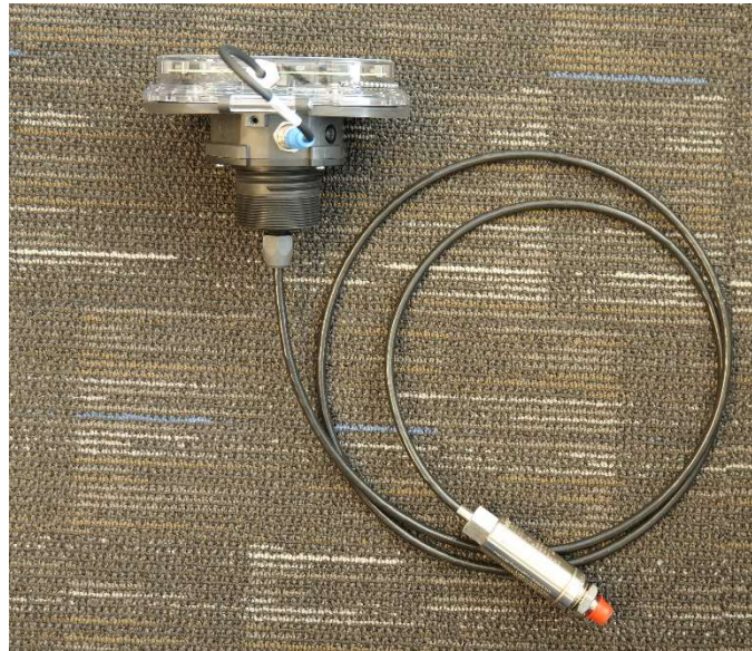
Figure 1: ST100 Gateway unit mounted to sensor unit
