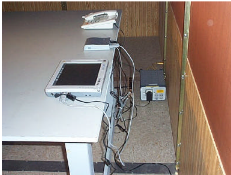
Conducted Emission Setup, showing cable placement
