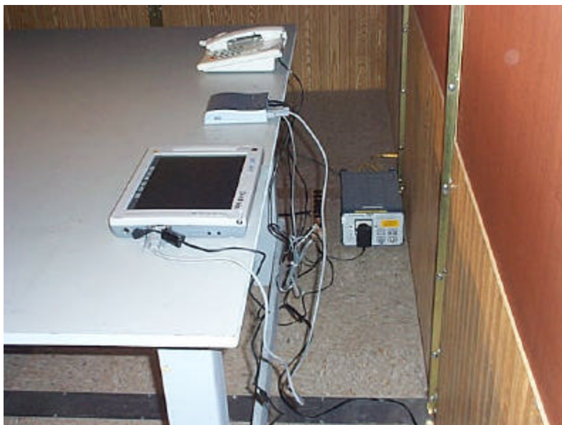
Conducted Emission Setup, showing cable placement
