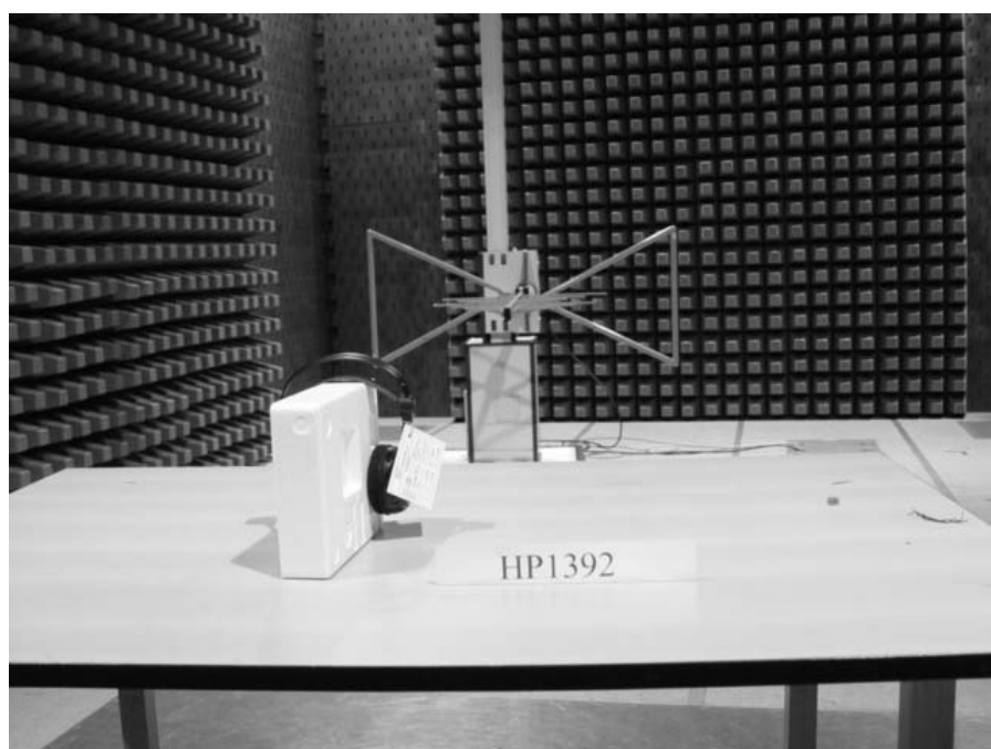
Photograph 2: Set-up for Radiation Measurement Below 1GHz
