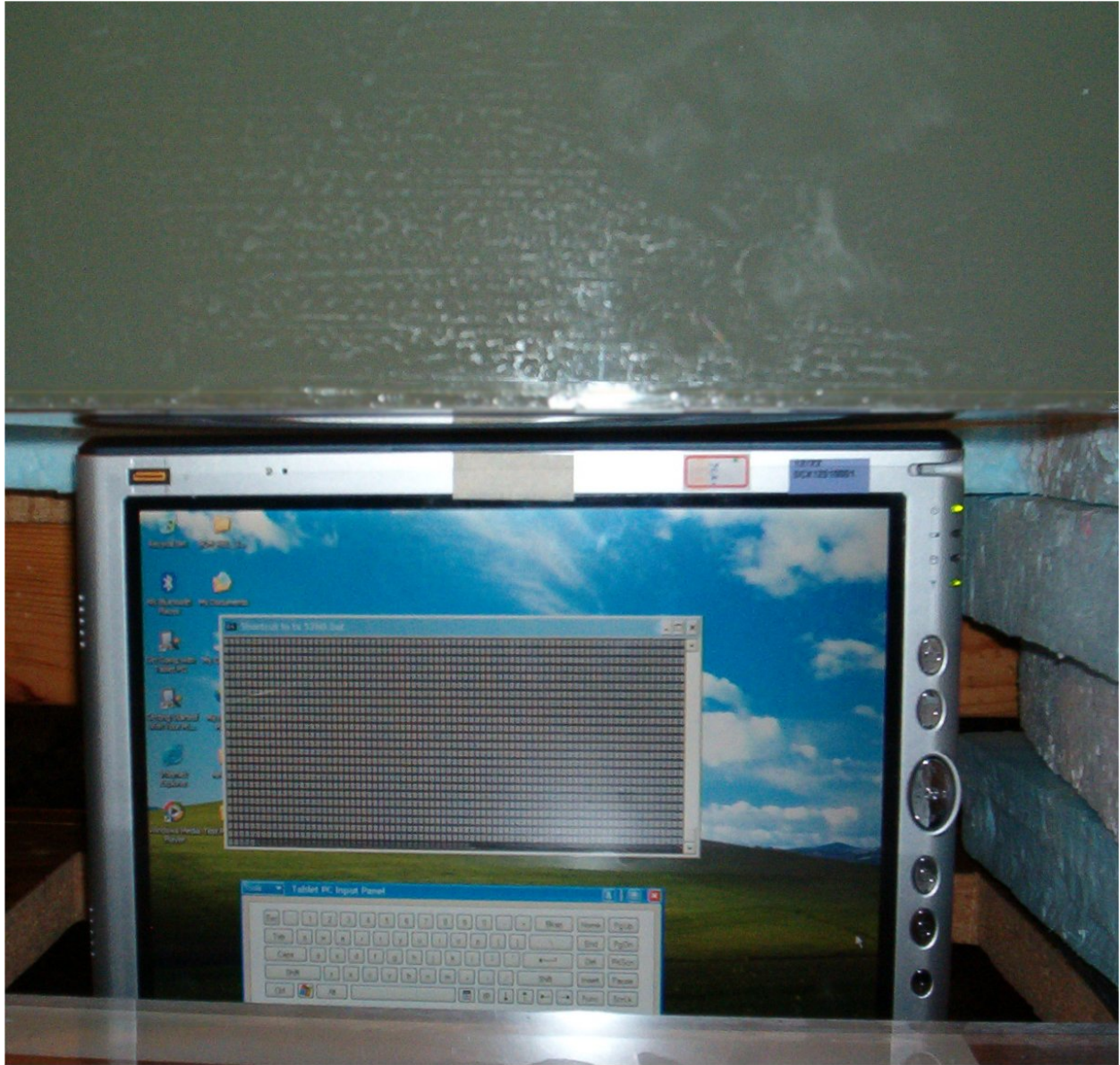
Fig. 2. Photograph of the Gemtek Technology Corporation Tablet PC at 90^\circ with the longer edge pressed against the bottom of the planar phantom. This is Edge-On Configuration 1 for SAR testing that corresponds to the longer edge of the Tablet PC pressed against the chest.
