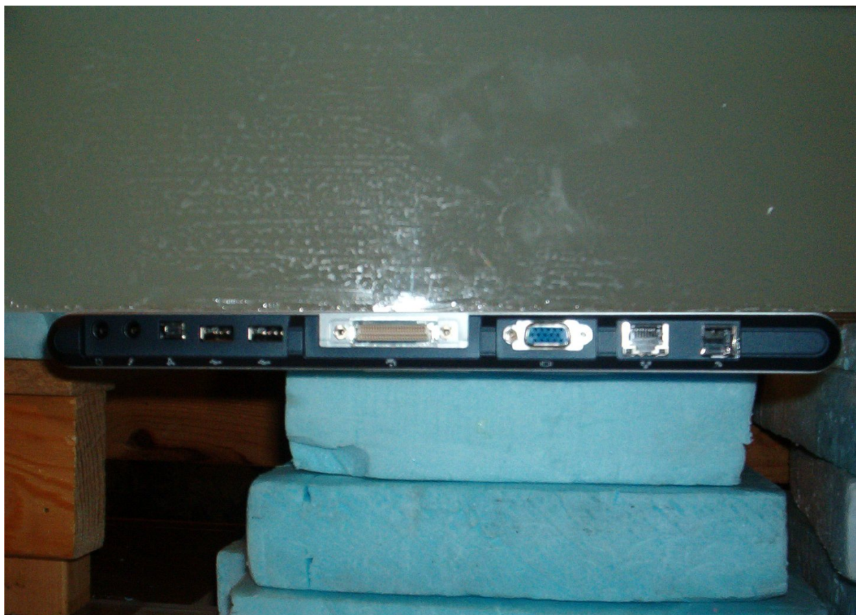
Fig. 4. Photograph of the bottom of the Gemtek Technology Corporation Tablet PC pressed against the bottom of the planar phantom. This is Configuration 3 – Above-Lap Position for SAR testing.
