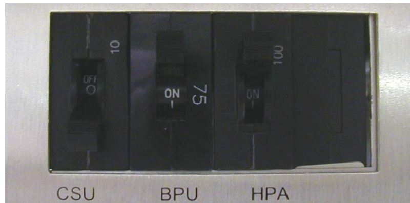
Figure 1-8 Circuit Breakers on Front Panel of BTS-4000
