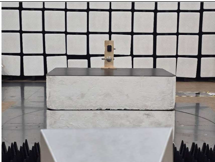
[Rear view of Radiated Emission (Above 1GHz)]_ YMC654-4(Alt. Model)
