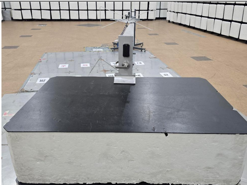
[Rear view of Radiated Emission (Below 1GHz)]_ YMC614-5.5(Alt. Model)
