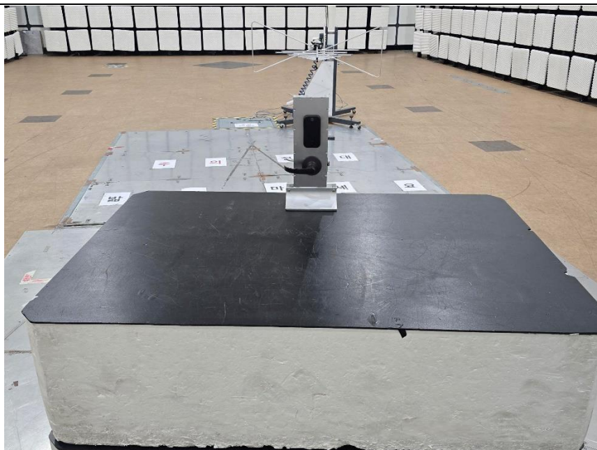
[Rear view of Radiated Emission (Below 1GHz)]_ YMC624-5.5(Basic Model)
