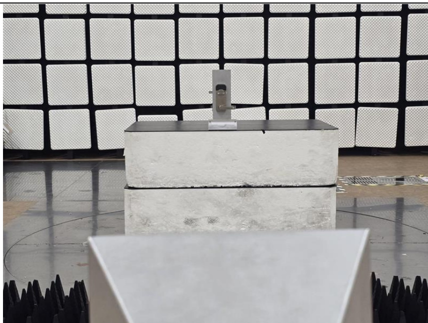
[Rear view of Radiated Emission (Above 1GHz)]_ YMC624-5.5(Basic Model)
