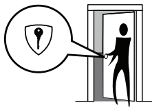
Right Hand " RH ", Hinges Right. Open Inward.
