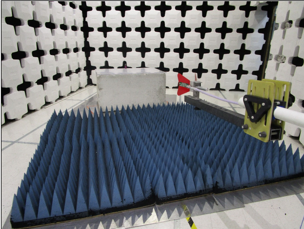
Test Setup for Radiated Emissions: 1GHz to 13GHz, Horizontal Polarization
