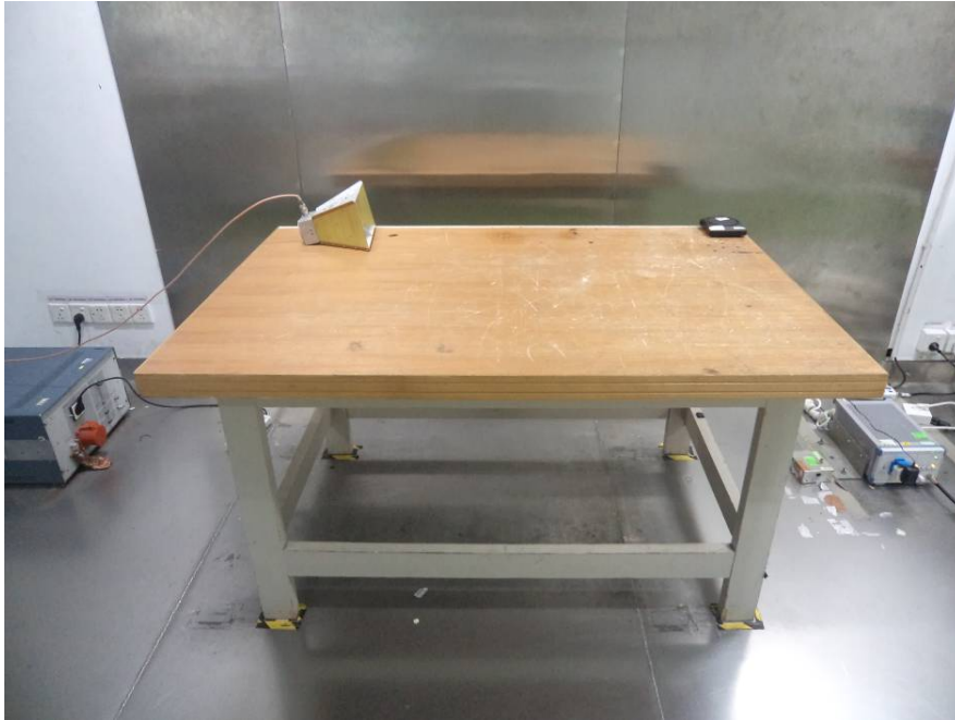
Conducted Emissions - Front View
