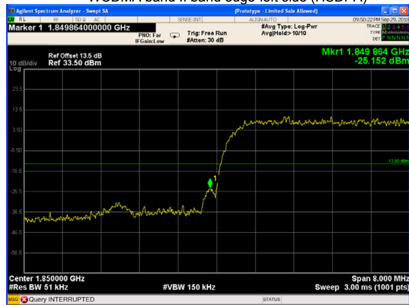
WCDMA band II band edge-left side (HSDPA)
