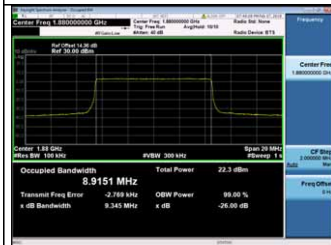
LTE band 2 - Low CH QPSK-10
