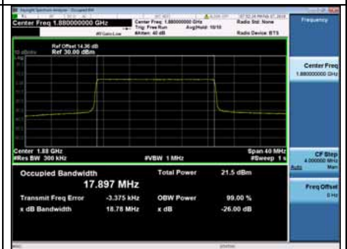
LTE band 2 - Low CH 16QAM-20
