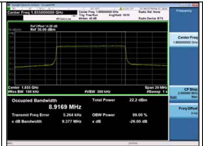
LTE band 2 - Low CH 16QAM-10
