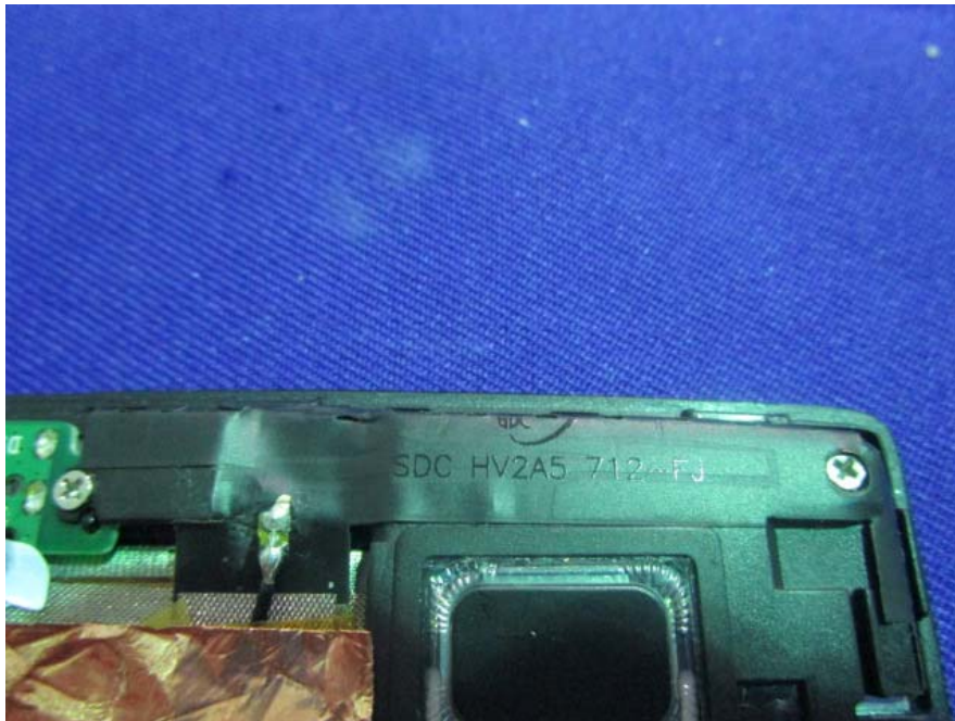
EUT –GSM&WCDMA Antenna View
