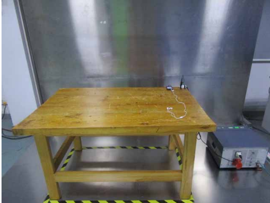
Conducted Emission – Front View
