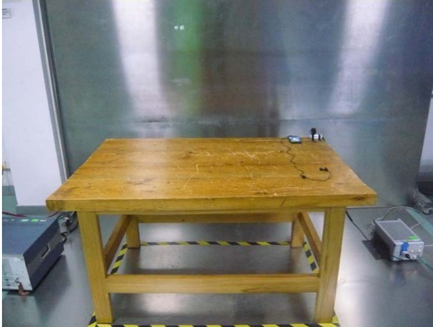
Conducted Emission- Front View
