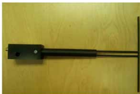
Figure 1 – MVG COMOSAR Validation Dipole
