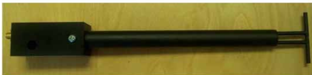
Figure 1 – MVG COMOSAR Validation Dipole
