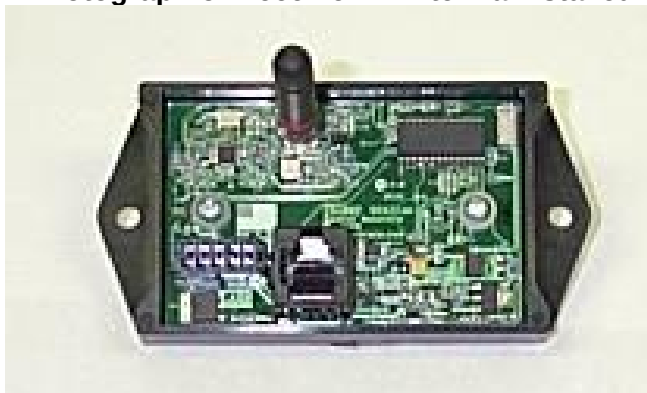
Photograph of Receiver – Antenna Installed
