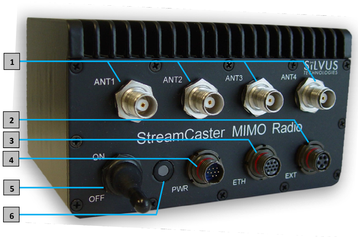
Figure 3 StreamCaster 3500/3800 Ruggedized Enclosure
