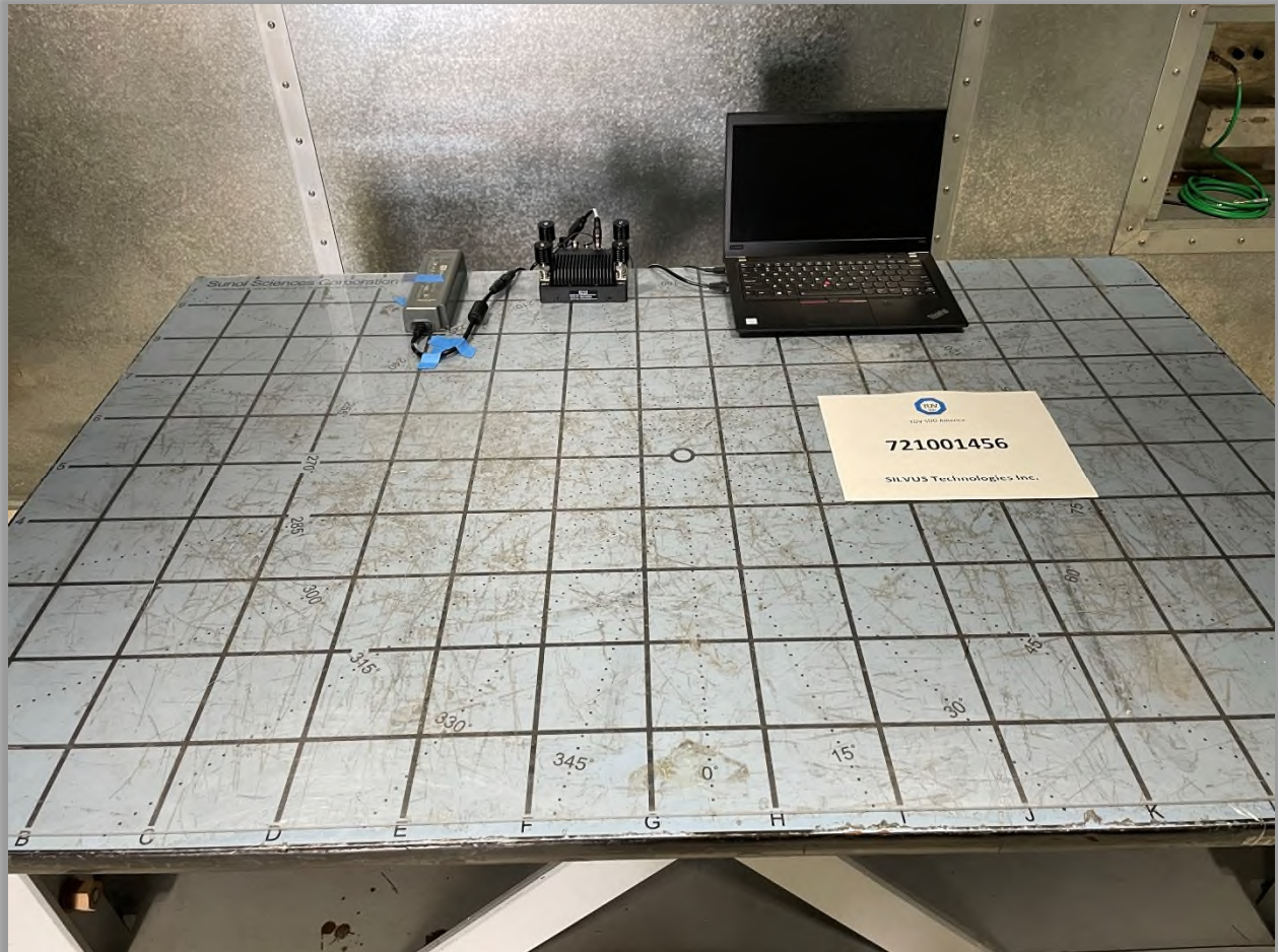
Conducted Emissions Back Front Test Setup
