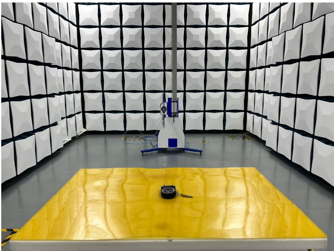
Set up for Radiated Emission Below 200M~1G
