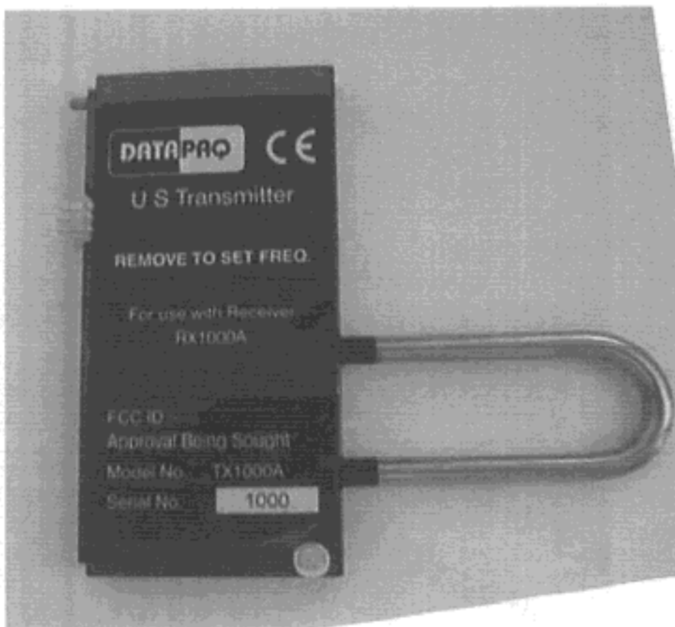
Exhibit 1: Rear view of transmitter showing design of product label and its location.
