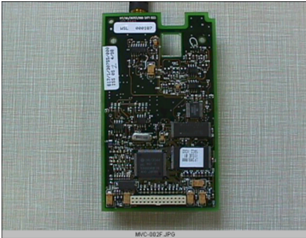
GPT Modem - Close Up of RF PCB Component Side
