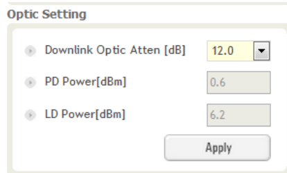
Figure 8-57 Optic Setting (Control - RU)
