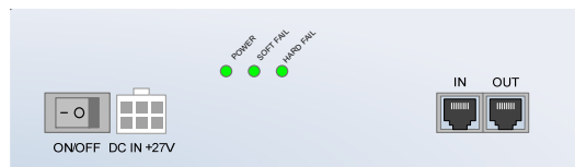
Figure 3-31 Ports at the rear panel (Slave RU)
