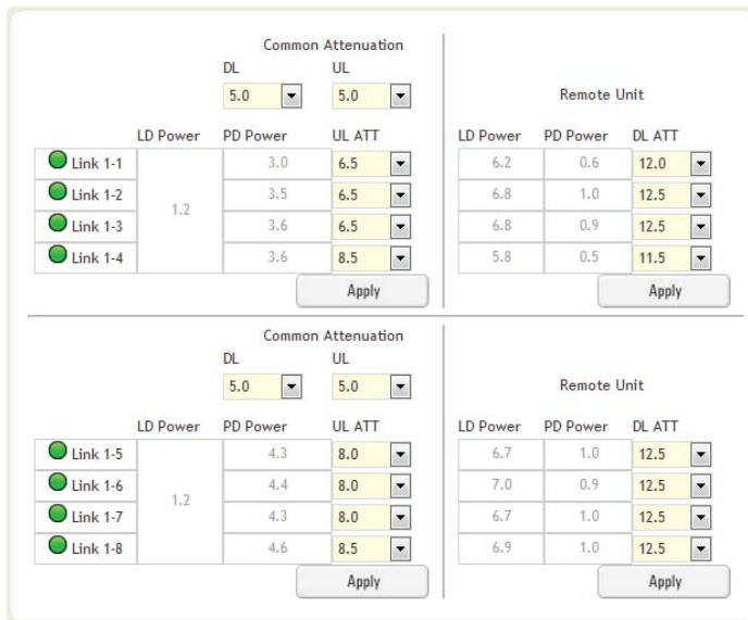
Figure 8-50 Optic Attenuation – OPT
