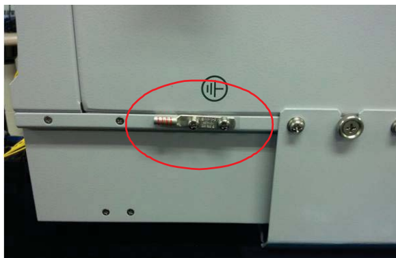
Figure 6-6 Ground Cable Connection (HRU dual side)
