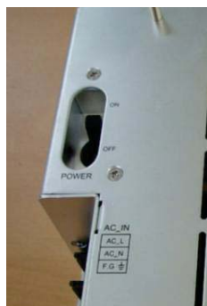
Figure 3-31 HRU AC Switch
