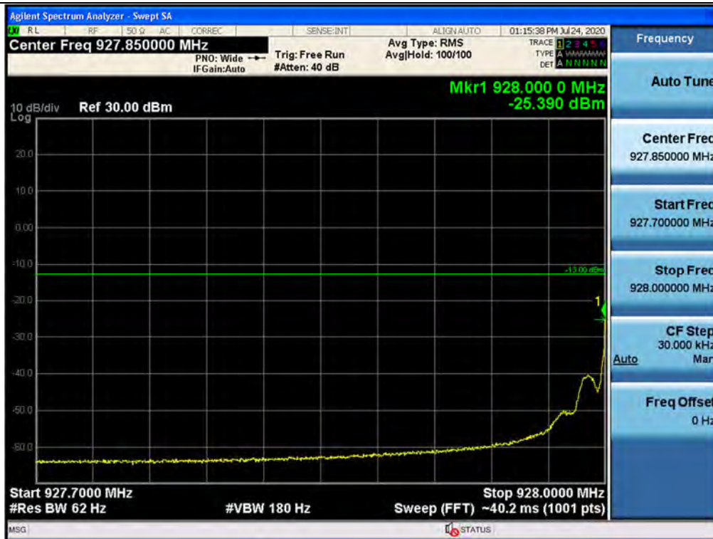
Out-of-band (two adjacent test signals) / 928 ~ 929 MHz / Downlink / P25 Phase 2 / Lower
