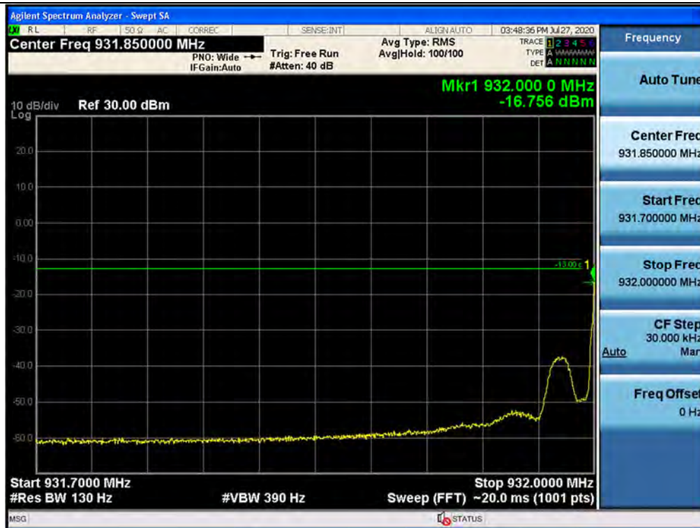
Out-of-band (two adjacent test signals) / 932 ~ 935 MHz / Downlink / P25 Phase 1 / Lower
