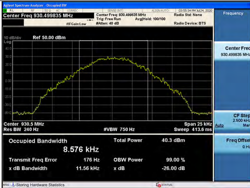
3 dB above the AGC threshold output / 930 ~ 931 MHz / Downlink / P25 Phase 1
