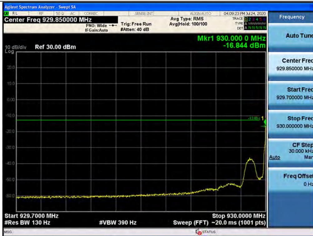
Out-of-band (two adjacent test signals) / 930 ~ 931 MHz / Downlink / P25 Phase 1 / Lower
