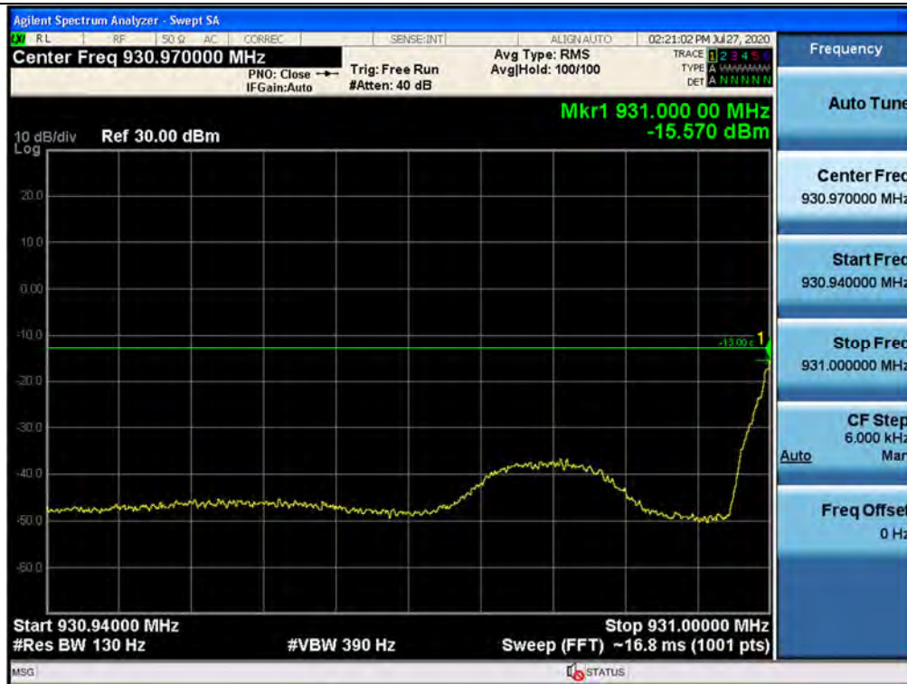
Out-of-band (two adjacent test signals) / 931 ~ 932 MHz / Downlink / P25 Phase 1 / Lower
