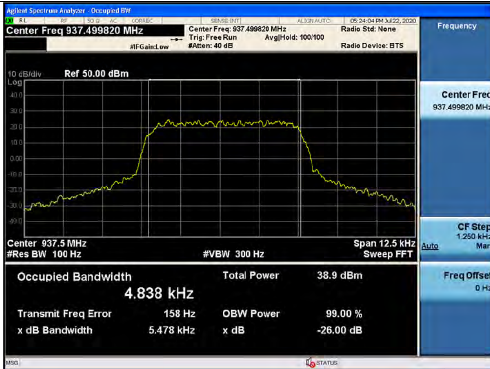
3 dB above the AGC threshold output / 935 ~ 940 MHz / Downlink / P25 Phase 2
