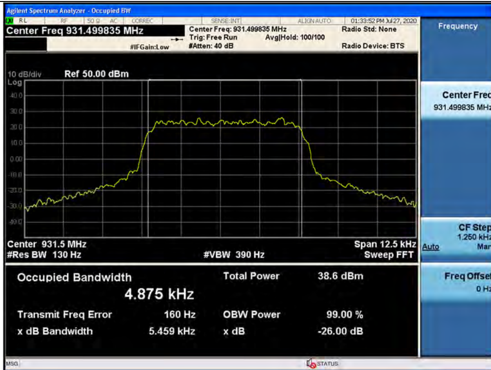
3 dB above the AGC threshold output / 931 ~ 932 MHz / Downlink / P25 Phase 2
