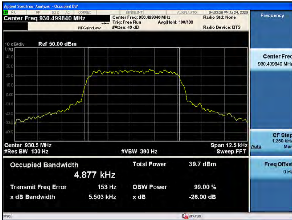
3 dB above the AGC threshold output / 930 ~ 931 MHz / Downlink / P25 Phase 2
