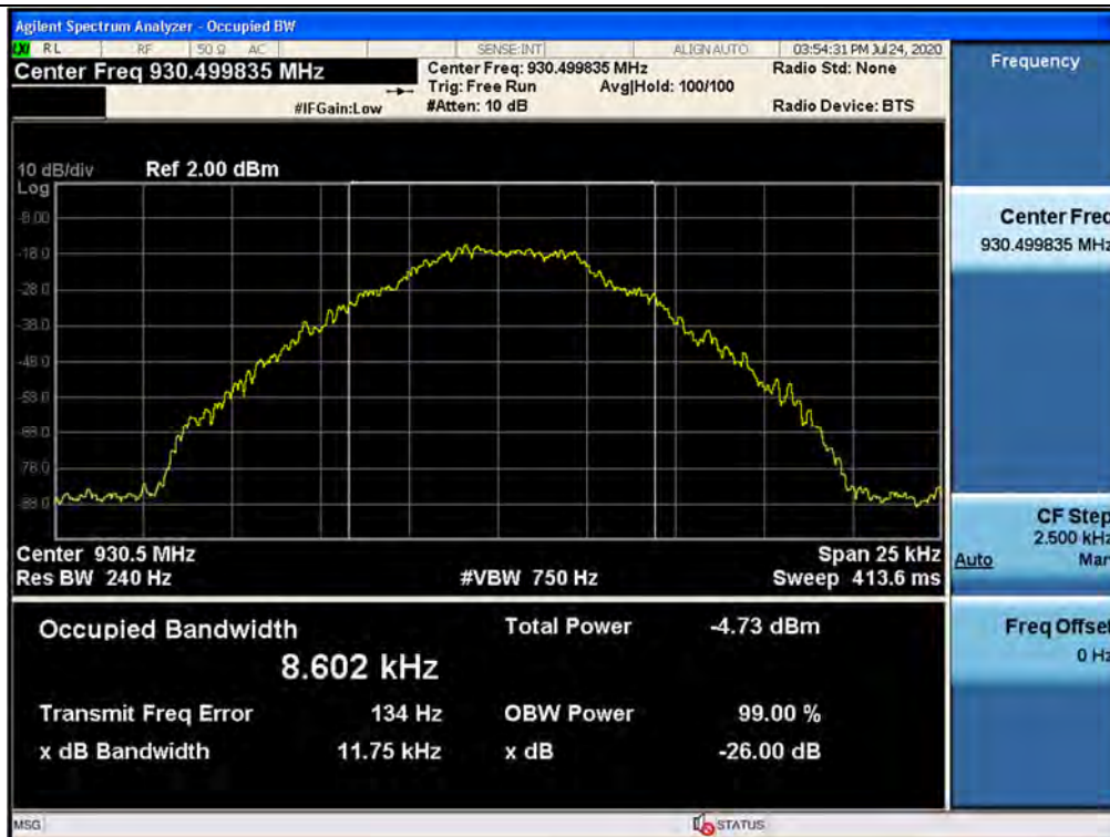
3 dB above the AGC threshold Input / 930 ~ 931 MHz / Downlink / P25 Phase 1
