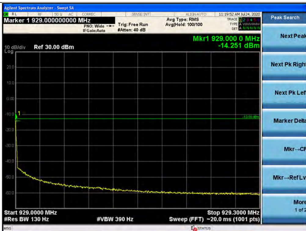
Out-of-band (single test signals) / 928 ~ 929 MHz / Downlink / P25 Phase 1 / Upper
