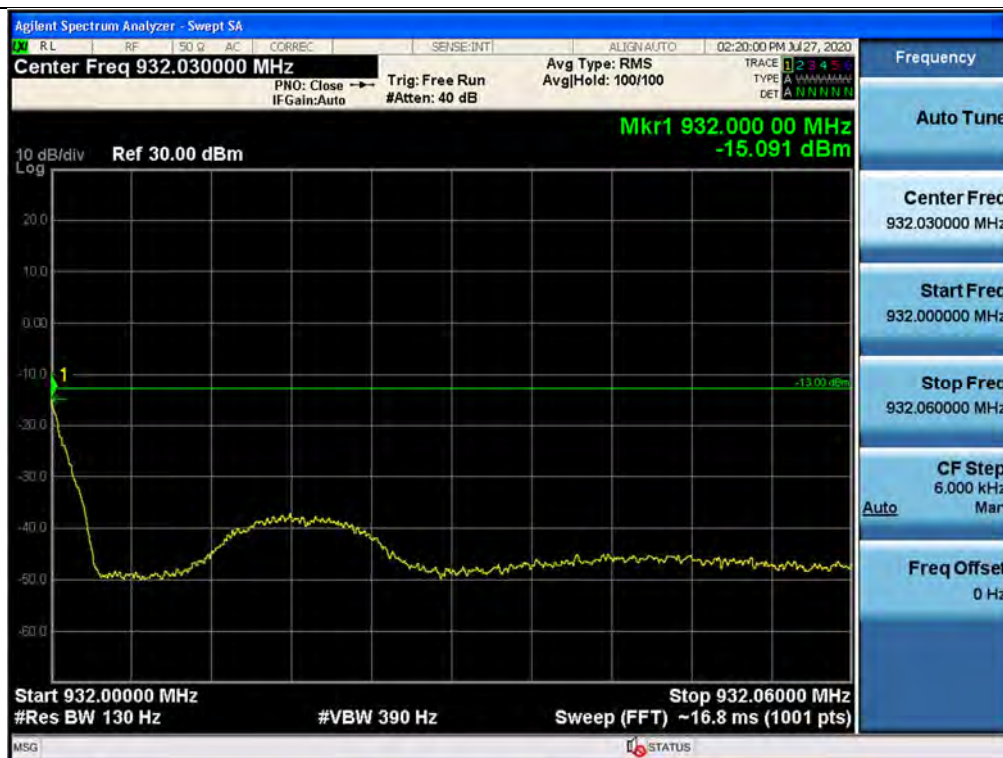
Out-of-band (two adjacent test signals) / 931 ~ 932 MHz / Downlink / P25 Phase 1 / Upper
