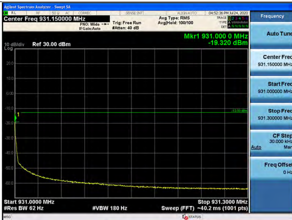
Out-of-band (single test signals) / 930 ~ 931 MHz / Downlink / P25 Phase 2 / Upper
