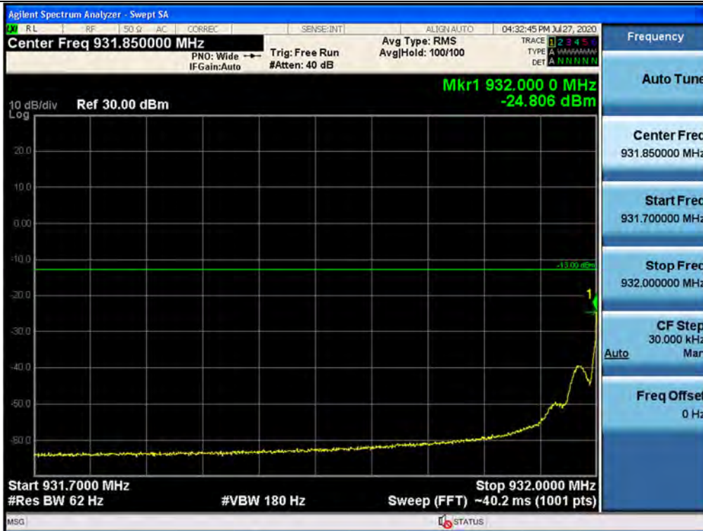
Out-of-band (two adjacent test signals) / 932 ~ 935 MHz / Downlink / P25 Phase 2 / Lower
