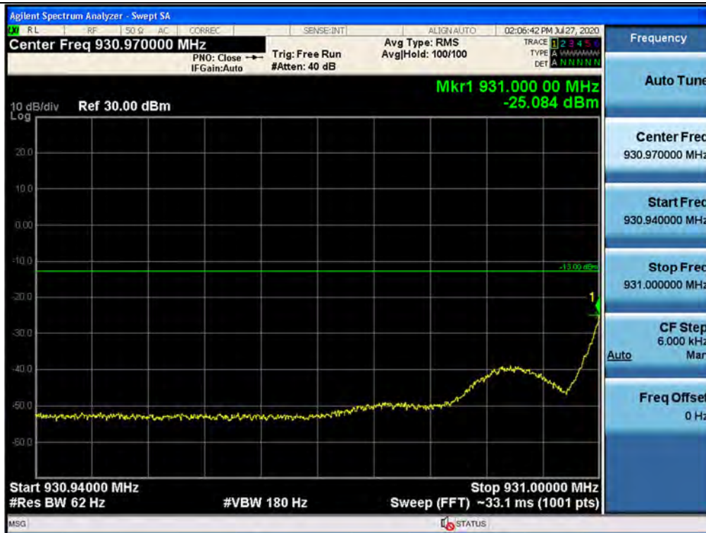
Out-of-band (two adjacent test signals) / 931 ~ 932 MHz / Downlink / P25 Phase 2 / Lower
