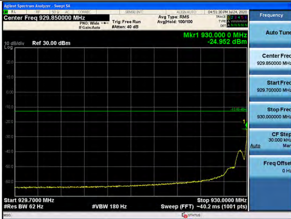
Out-of-band (two adjacent test signals) / 930 ~ 931 MHz / Downlink / P25 Phase 2 / Lower
