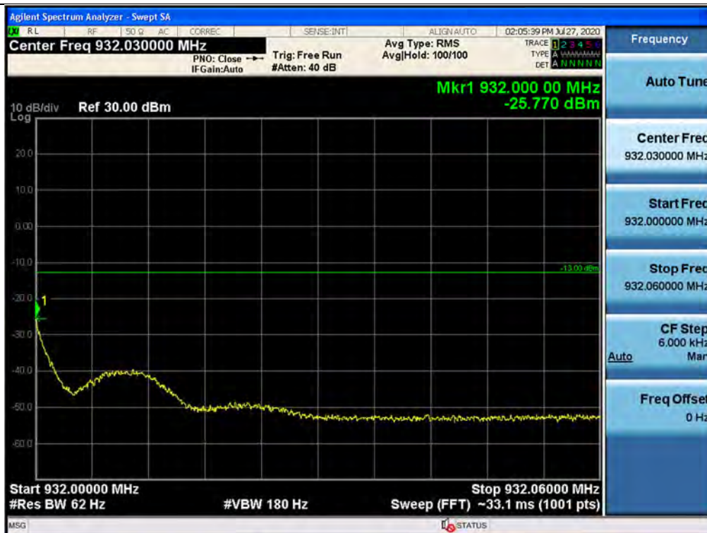
Out-of-band (two adjacent test signals) / 931 ~ 932 MHz / Downlink / P25 Phase 2 / Upper
