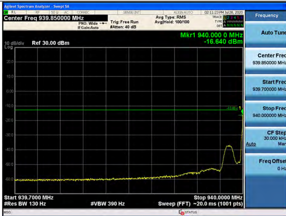
Out-of-band (two adjacent test signals) / 940 ~ 941 MHz / Downlink / P25 Phase 1 / Lower
