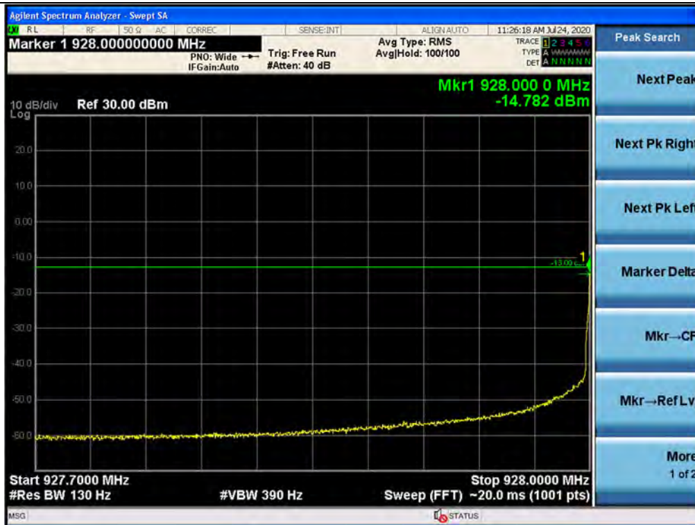
Out-of-band (single test signals) / 928 ~ 929 MHz / Downlink / P25 Phase 1 / Lower
