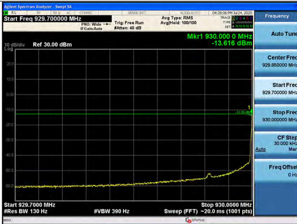
Out-of-band (single test signals) / 930 ~ 931 MHz / Downlink / P25 Phase 1 / Lower
