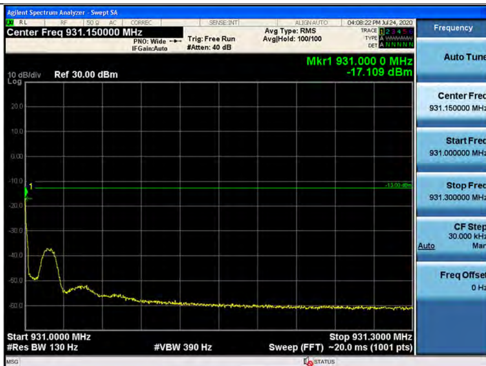
Out-of-band (two adjacent test signals) / 930 ~ 931 MHz / Downlink / P25 Phase 1 / Upper
