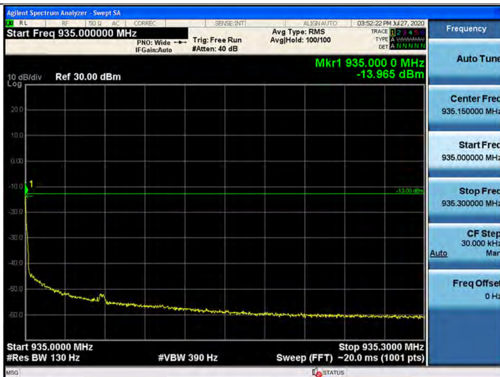
Out-of-band (single test signals) / 932 ~ 935 MHz / Downlink / P25 Phase 1 / Upper
