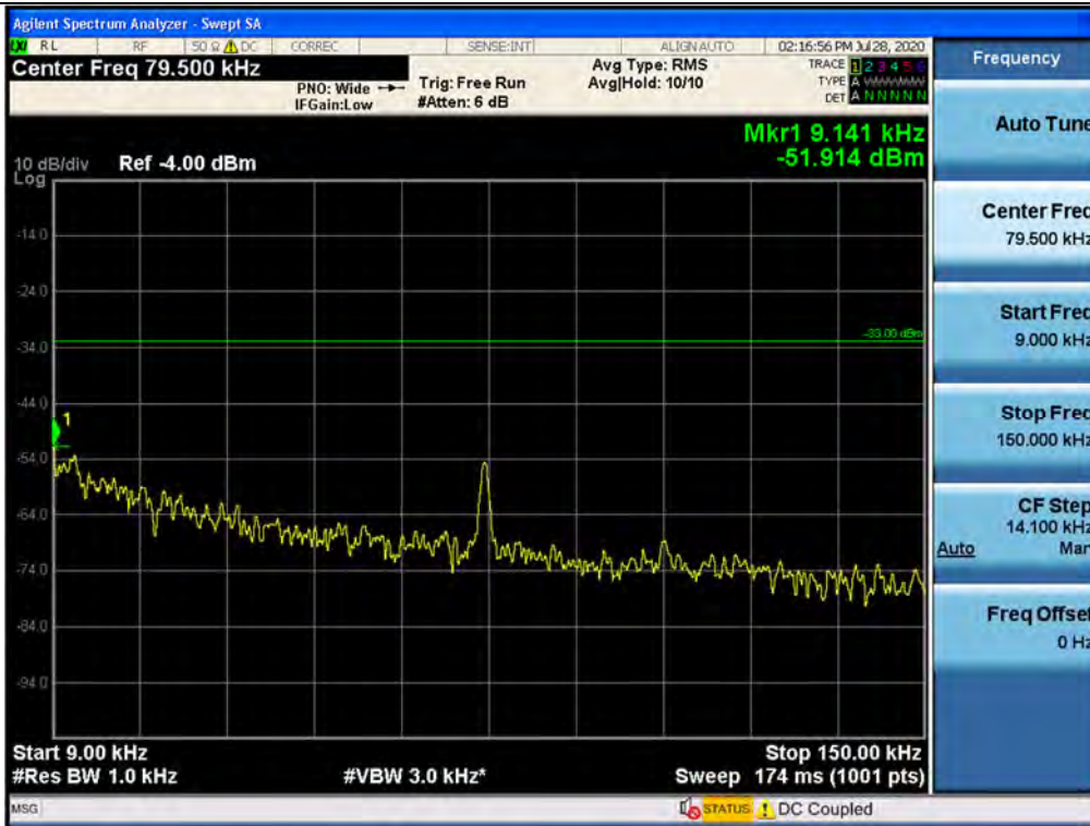
Spurious / 940 ~ 941 MHz / Downlink / P25 Phase 1 / Middle / 9 kHz ~ 150 kHz
