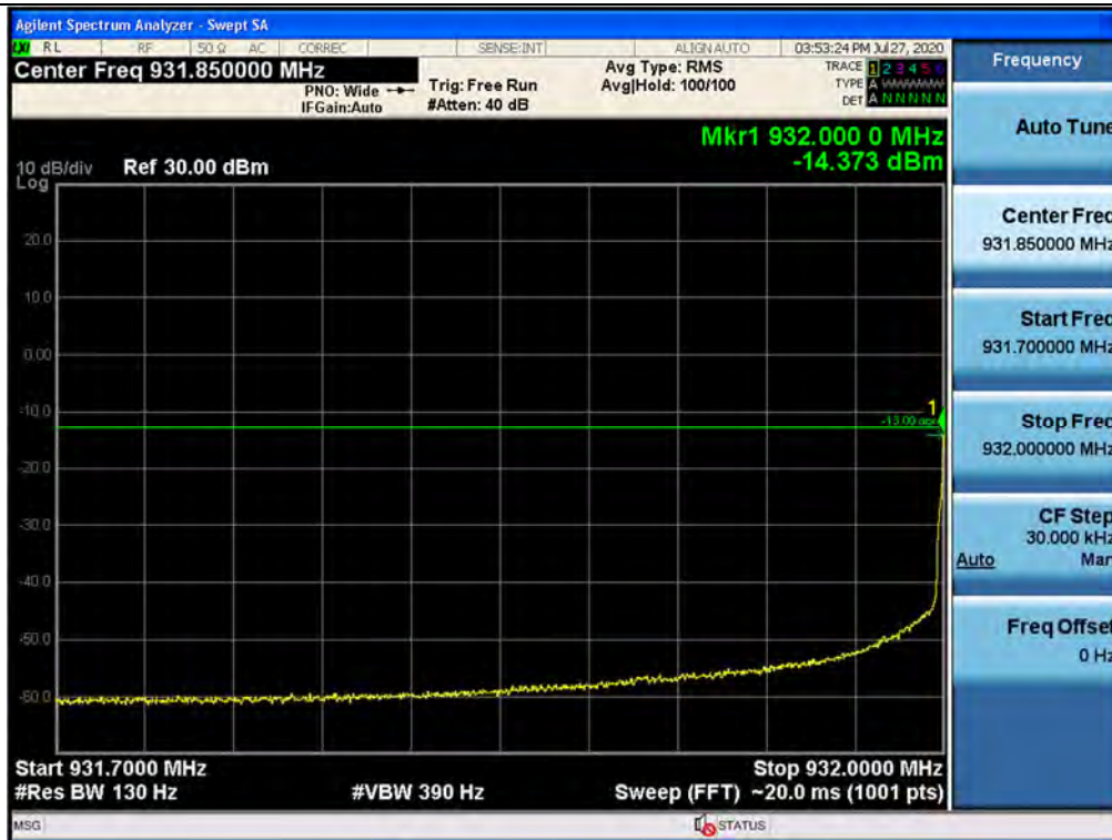
Out-of-band (single test signals) / 932 ~ 935 MHz / Downlink / P25 Phase 1 / Lower
