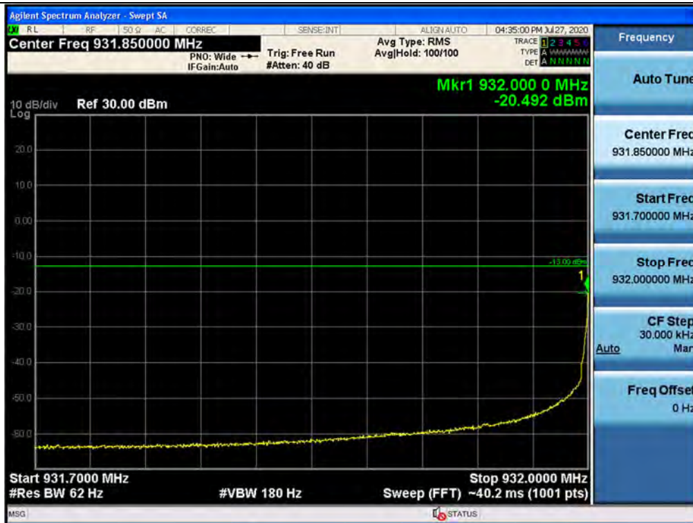
Out-of-band (single test signals) / 932 ~ 935 MHz / Downlink / P25 Phase 2 / Lower
