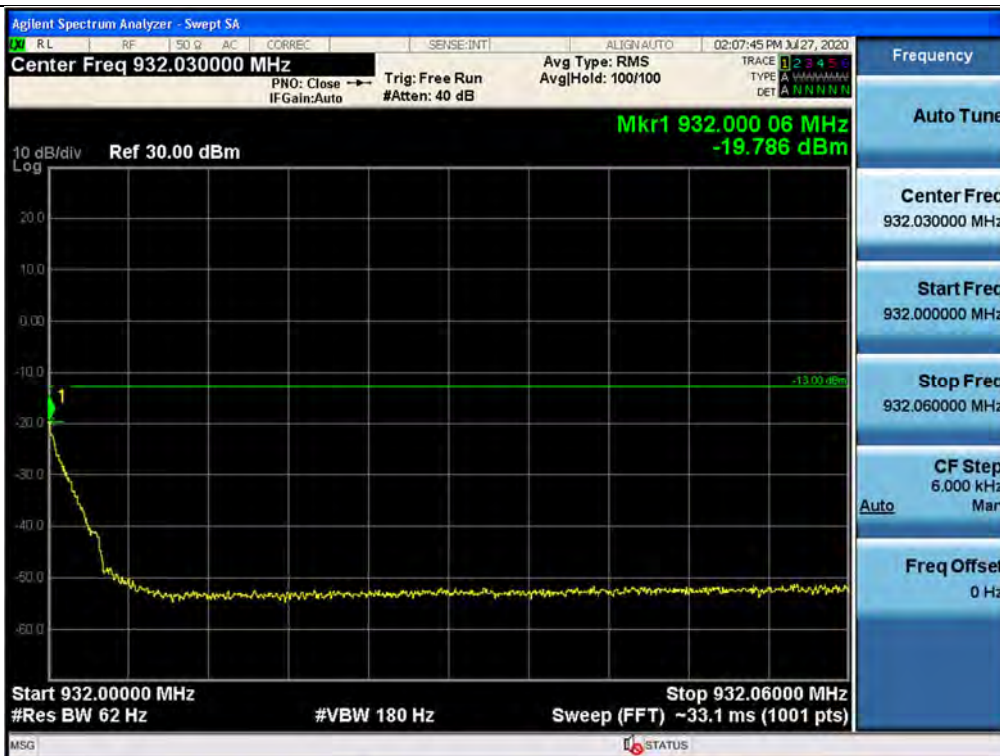
Out-of-band (single test signals) / 931 ~ 932 MHz / Downlink / P25 Phase 2 / Upper
