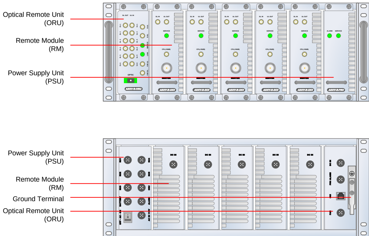
Figure 2-2 ADXV DAS RU Quick View (Front and Rear)
