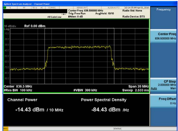
[SMR 800, Cellular AGC threshold Uplink LTE 10 MHz Mid]
