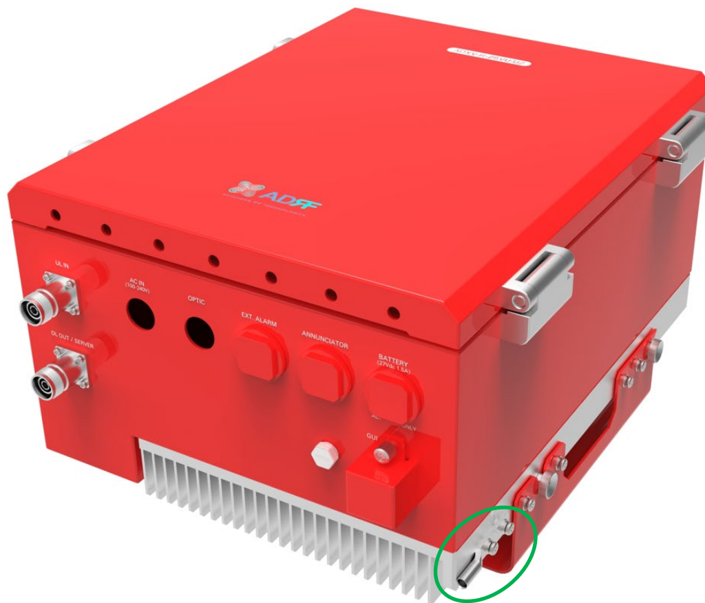
Figure 3-12 Protective Earthing Conductor
