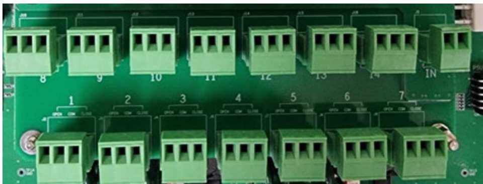
Figure 3-4 External Alarm port
