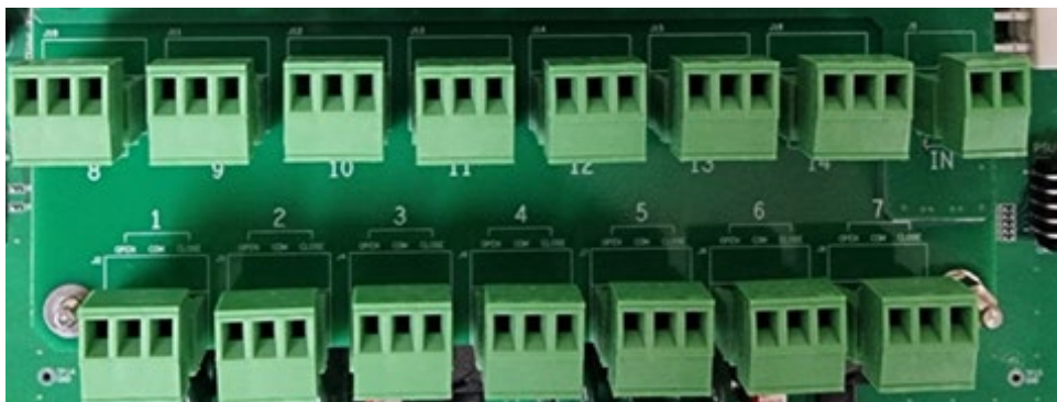
Figure 3-16 External Alarm port
