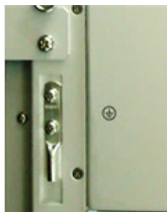
Figure 4-2 Ground Cable Connection
