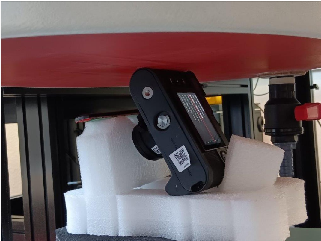
Photo 12: Test position left side without any distance with hand grip
