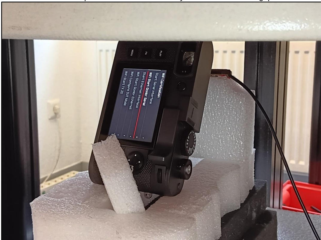
Photo 14: Test position left side without any distance with thumb grip black
