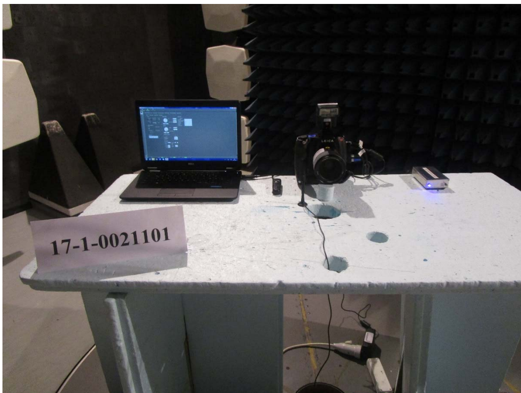
Photograph 2: Radiated measurements test set-up ( f < 1\text{GHz} )
