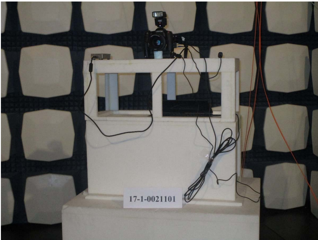
Photograph 4: Test set-up ( f > 1\text{GHz} )
