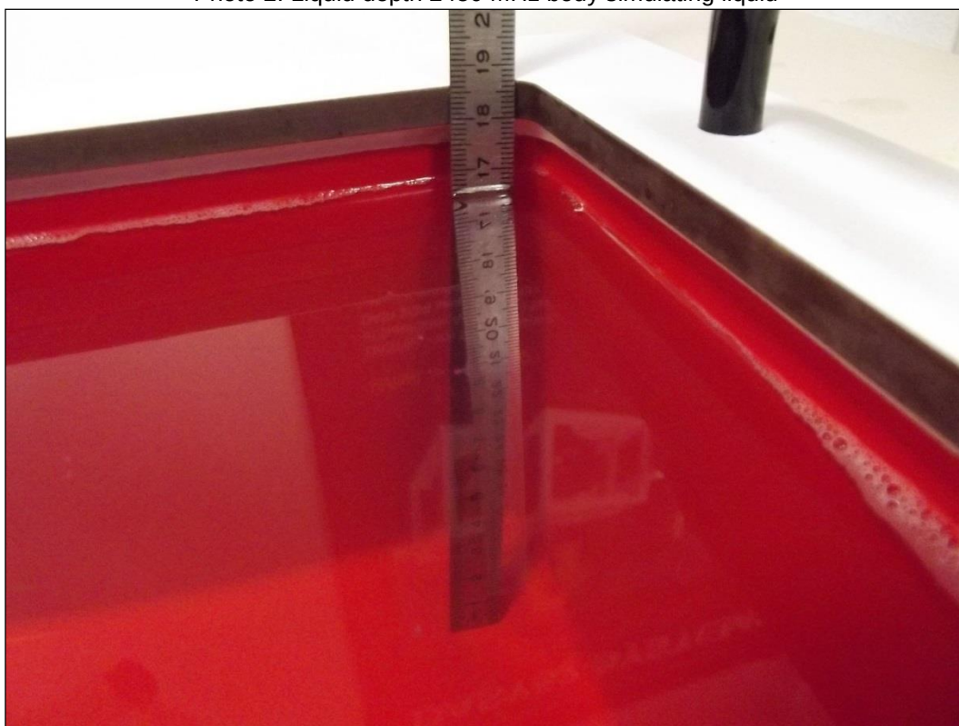
Photo 2: Liquid depth 2450 MHz body simulating liquid
