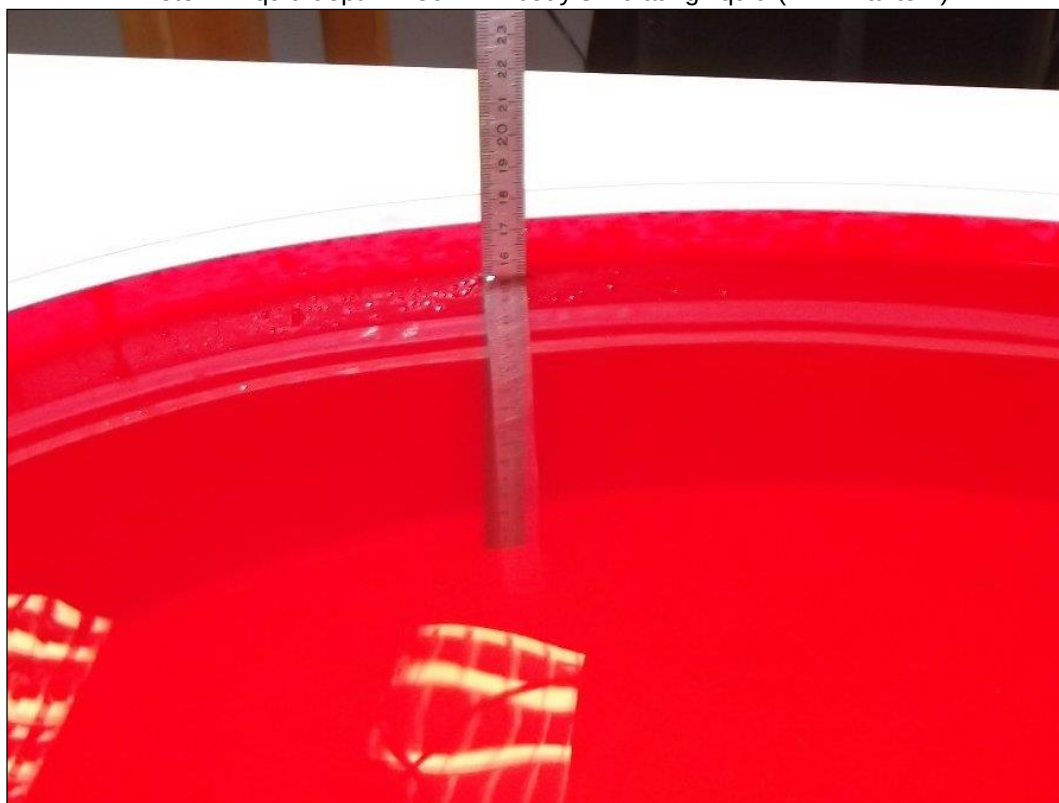
Photo 2: Liquid depth 2450 MHz body simulating liquid (ELI Phantom)
