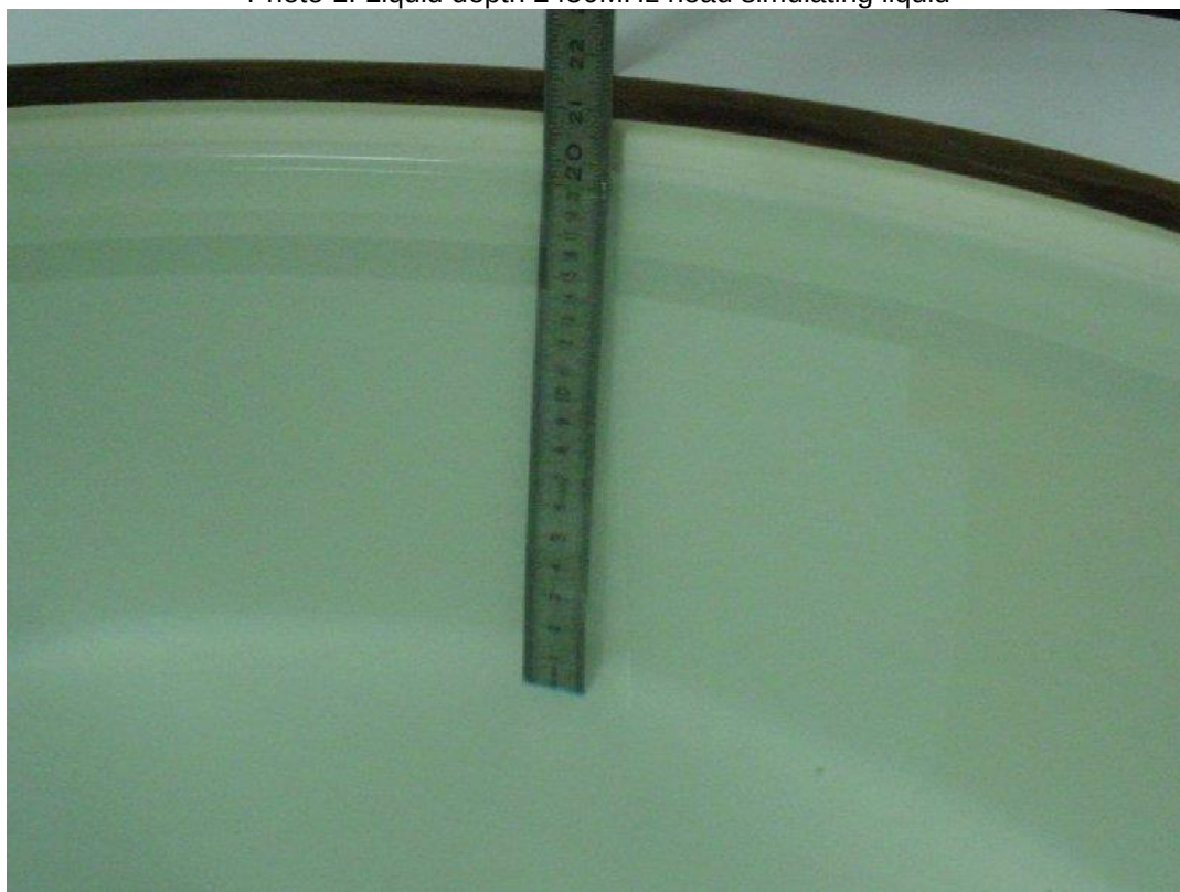
Photo 2: Liquid depth 2450 MHz body simulating liquid (ELI Phantom)
