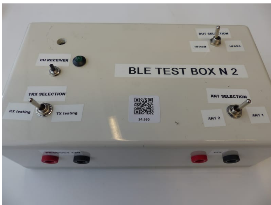
Photo 17: AE3: "BLE TEST BOX N 2" (for ISED only)
