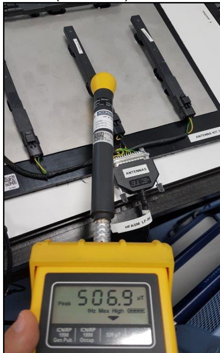
Photo 2: Test position - Antenna A (Dashboard) with ELT 400 3cm 2 probe (0mm distance)
