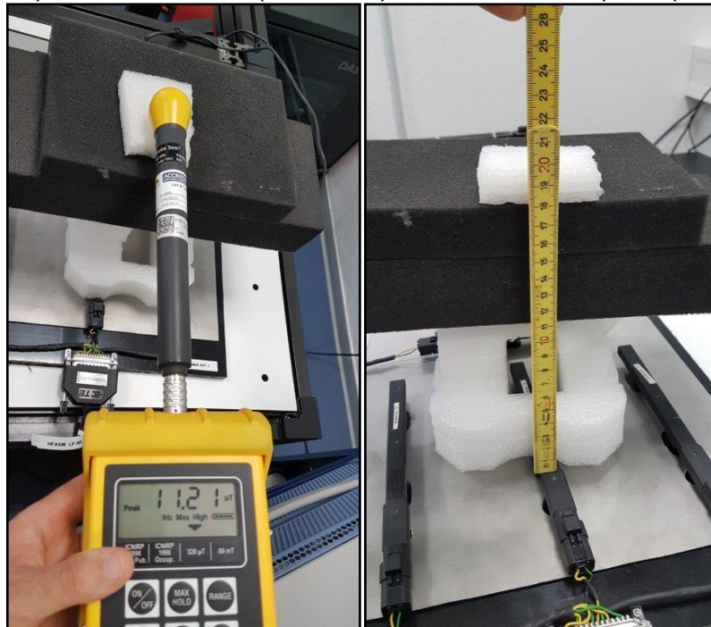
Photo 4: Test position - Antenna A (Dashboard) with HFH2-Z4 probe (3cm distance)
