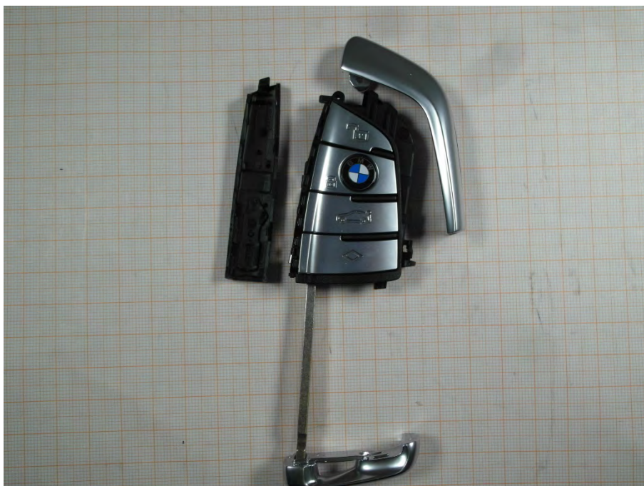
Photo 4: metal cover and button holder (left side) removed, EN version
