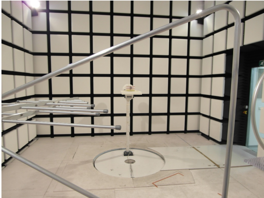
Photo 5: chrome variant 3m fully anechoic chamber
