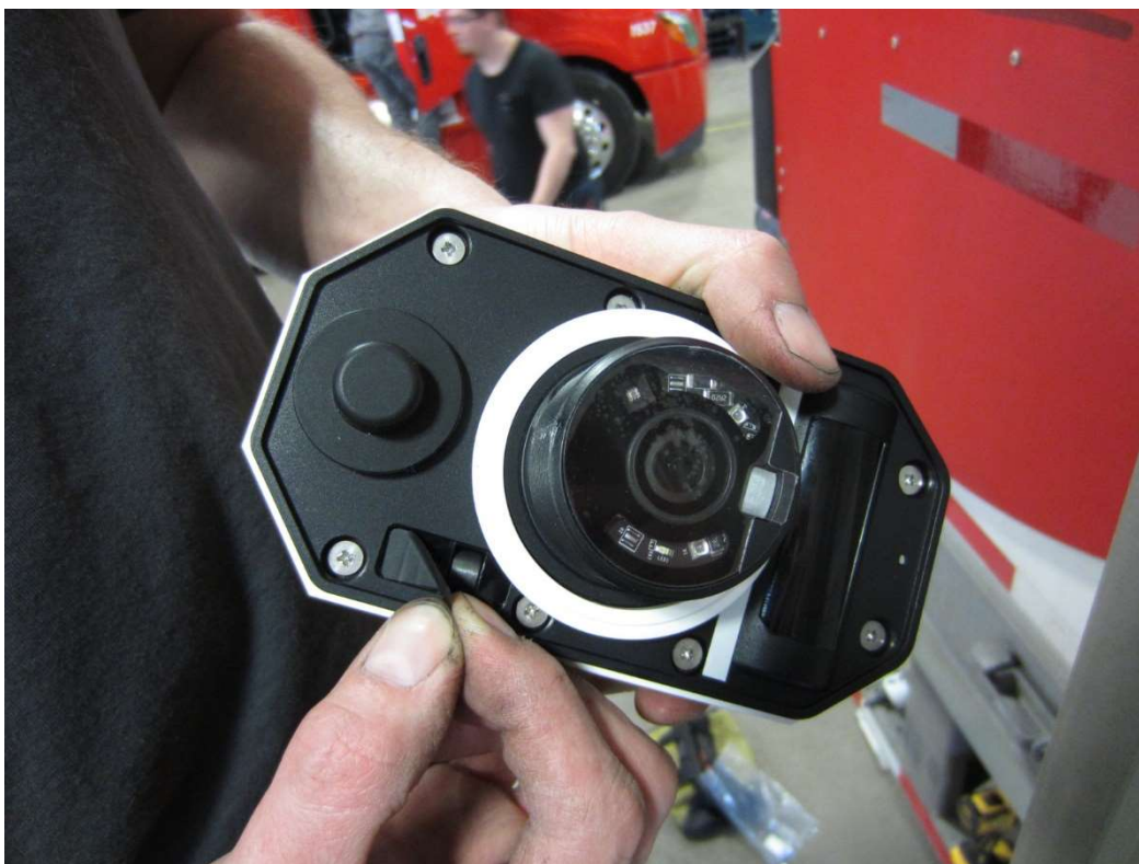
Removing tape over activation magnet
