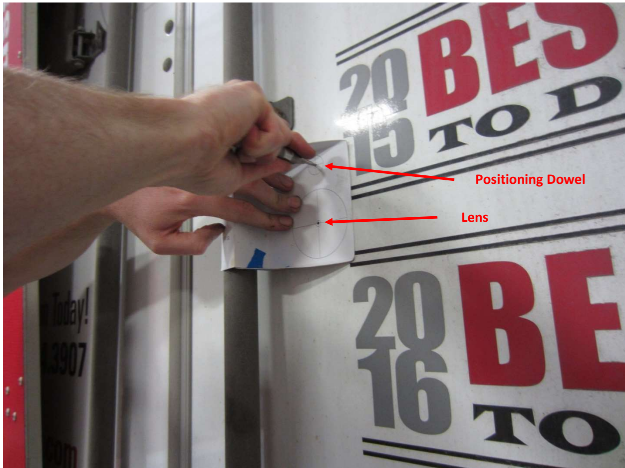
Mark hole locations with spring-loaded punch
