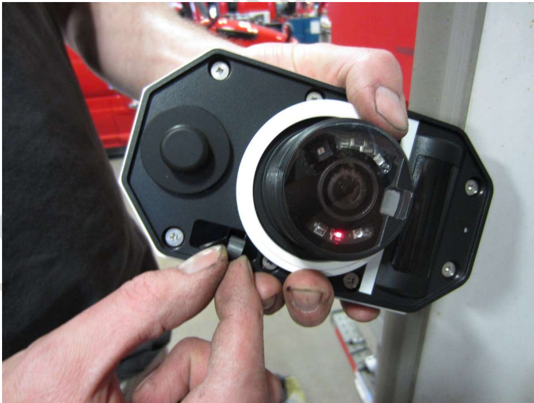
Activation magnet removal and LED flash
