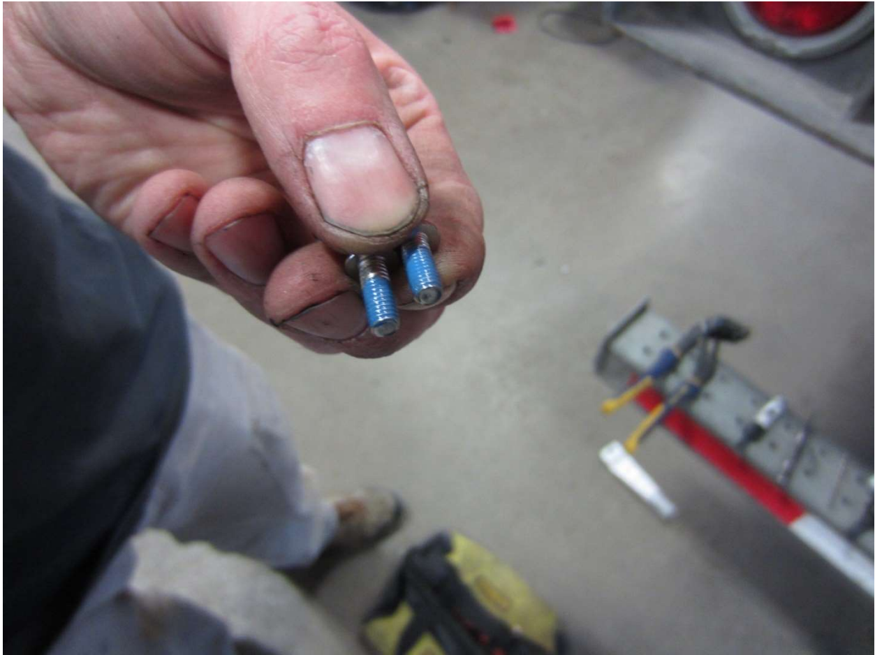
Loctite applied to thread forming screws
