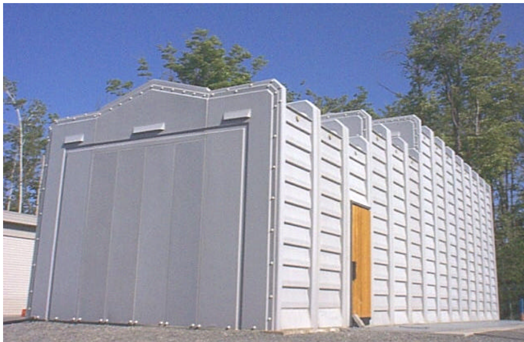
Fig. 7.b APREL's OATS(Open Area Test Site)
