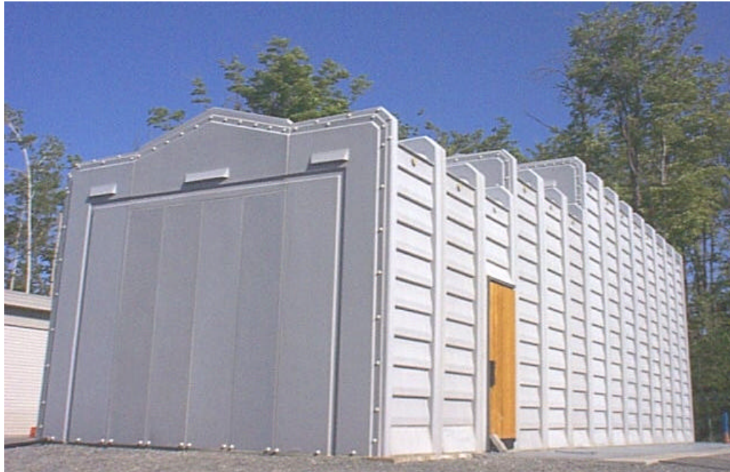
Fig. 1.b APREL's OATS (Open Area Test Site)
