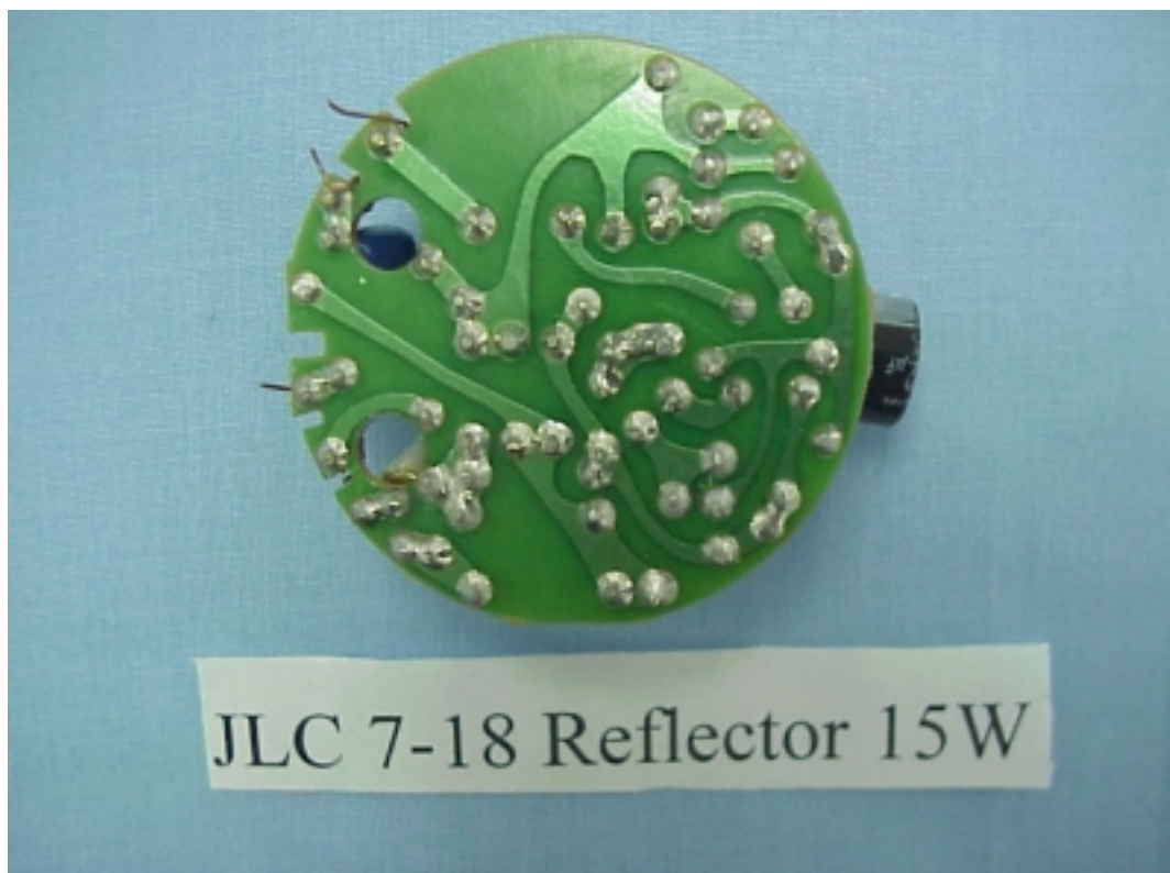
Figure 6 ENERGY SAVING LAMP (M/N: JLC 7-18 REFLECTOR 15W) MAIN BOARD (SOLDERED SIDE)
