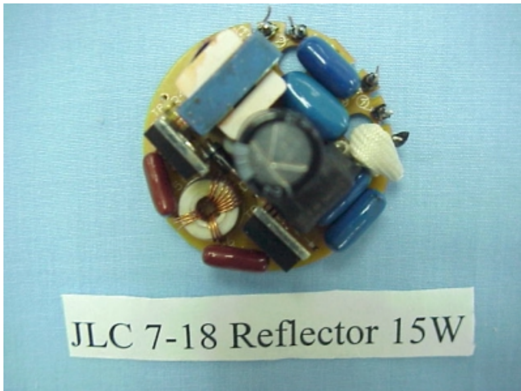
Figure 5 ENERGY SAVING LAMP (M/N: JLC 7-18 REFLECTOR 15W) Main Board (Component Side)
