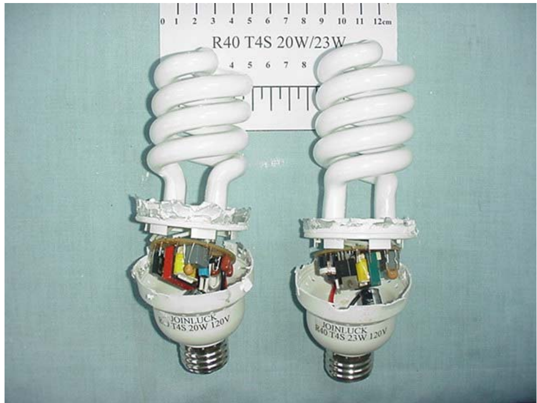
FIGURE 4 ENERGY SAVING LAMP (M/N: M/N: R40 T4S 20W/23W) COVER REMOVED
