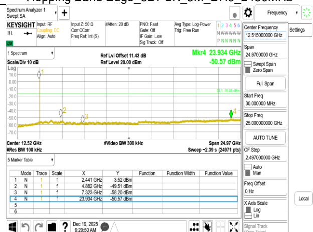
Spurious Emission GFSK 1M DH5 2441MHz
