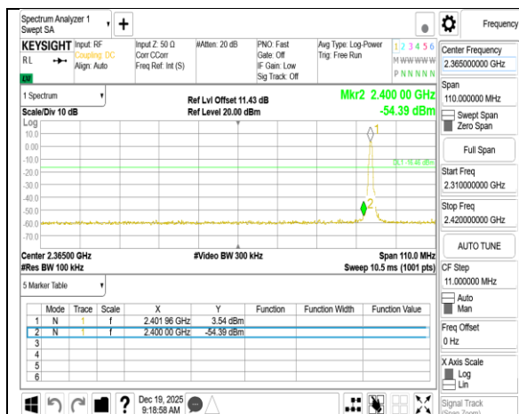
Band Edge_GFSK 1M DH5 2402MHz
