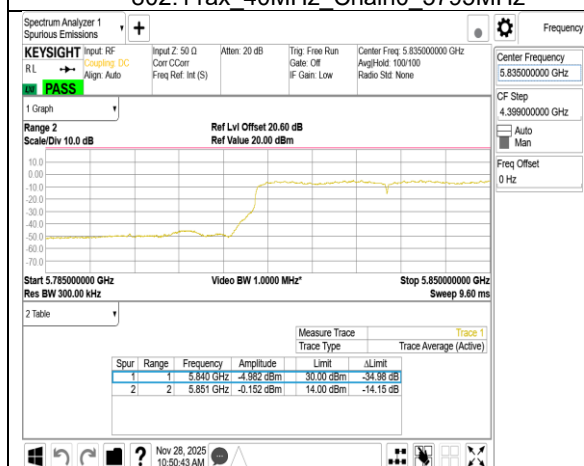
802.11ax 40MHz Chain0 5835MHz UNII 2C
