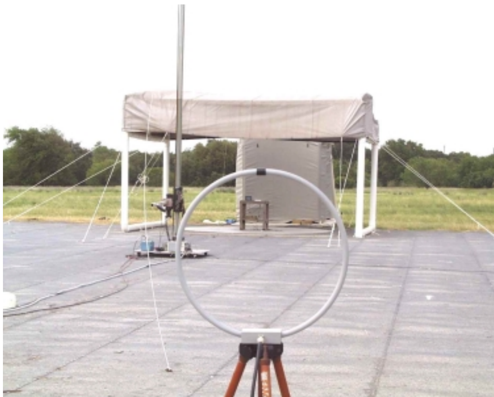
Radiated Emissions OATS Test Setup (110 kHz to 30 MHz)
