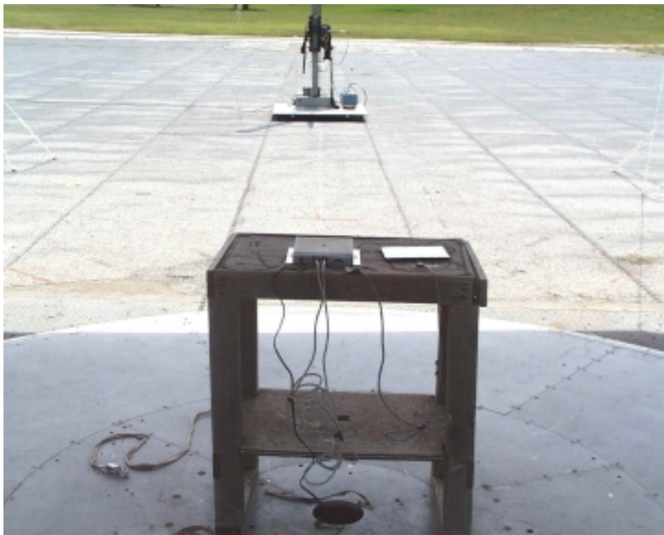
Radiated Emissions OATS Test Setup (30 MHz to 1 GHz)
