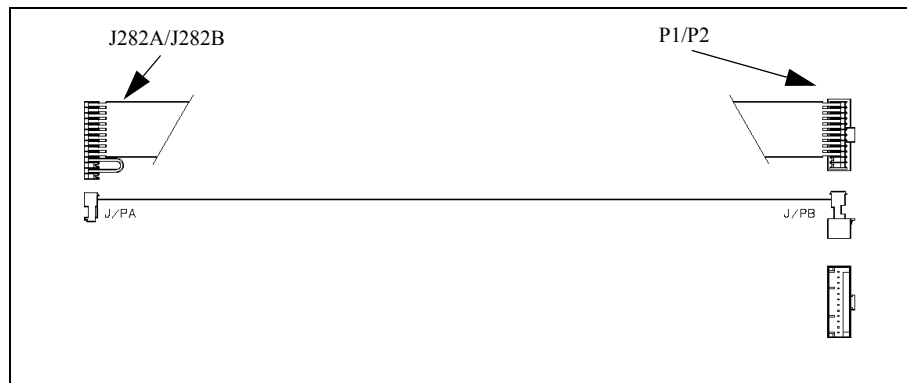
Figure 2: M00507A00X Ribbon Cable
