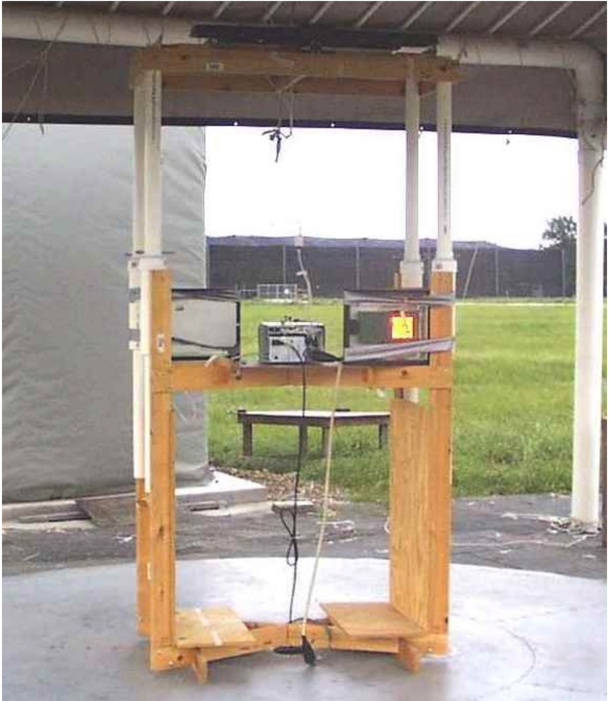
Radiated Emissions OATS Test Setup
