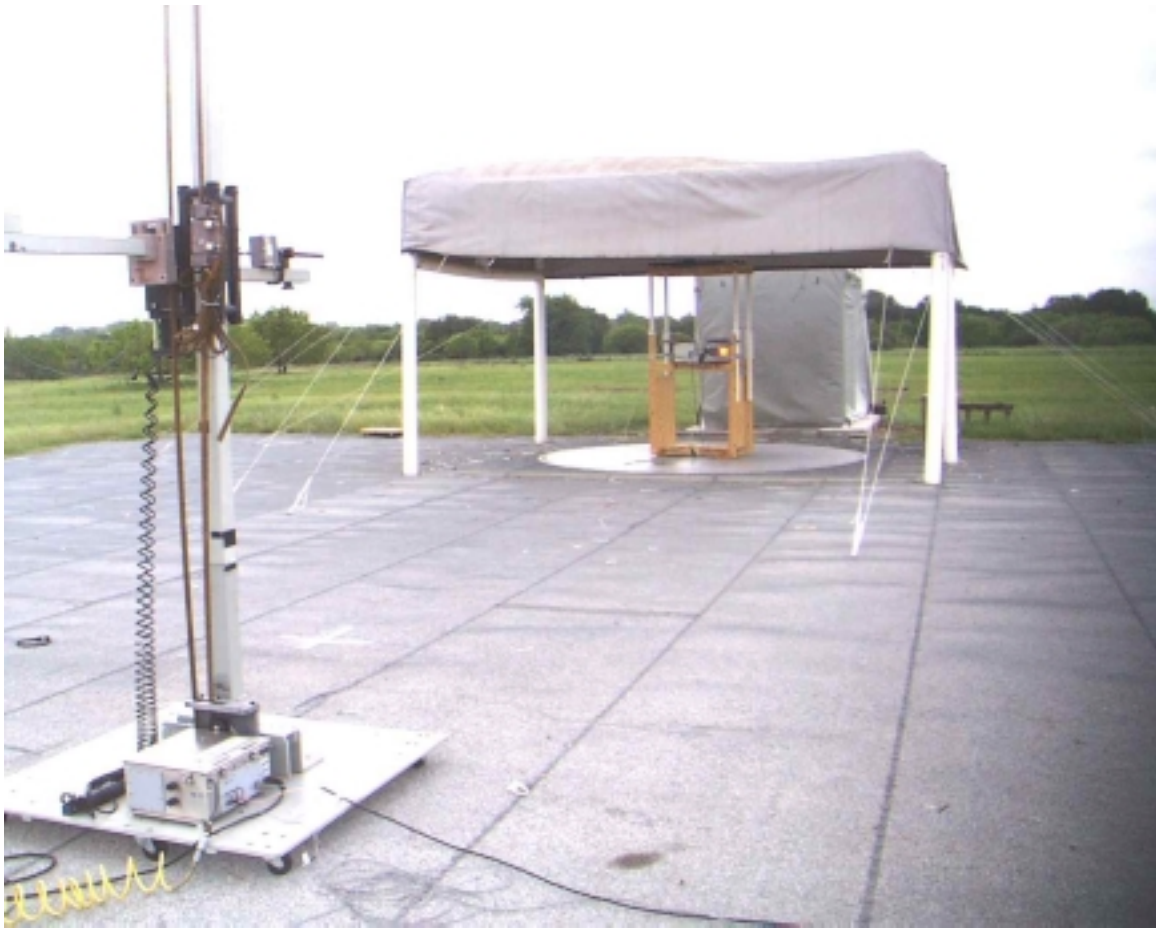
Radiated Emissions OATS Test Setup
