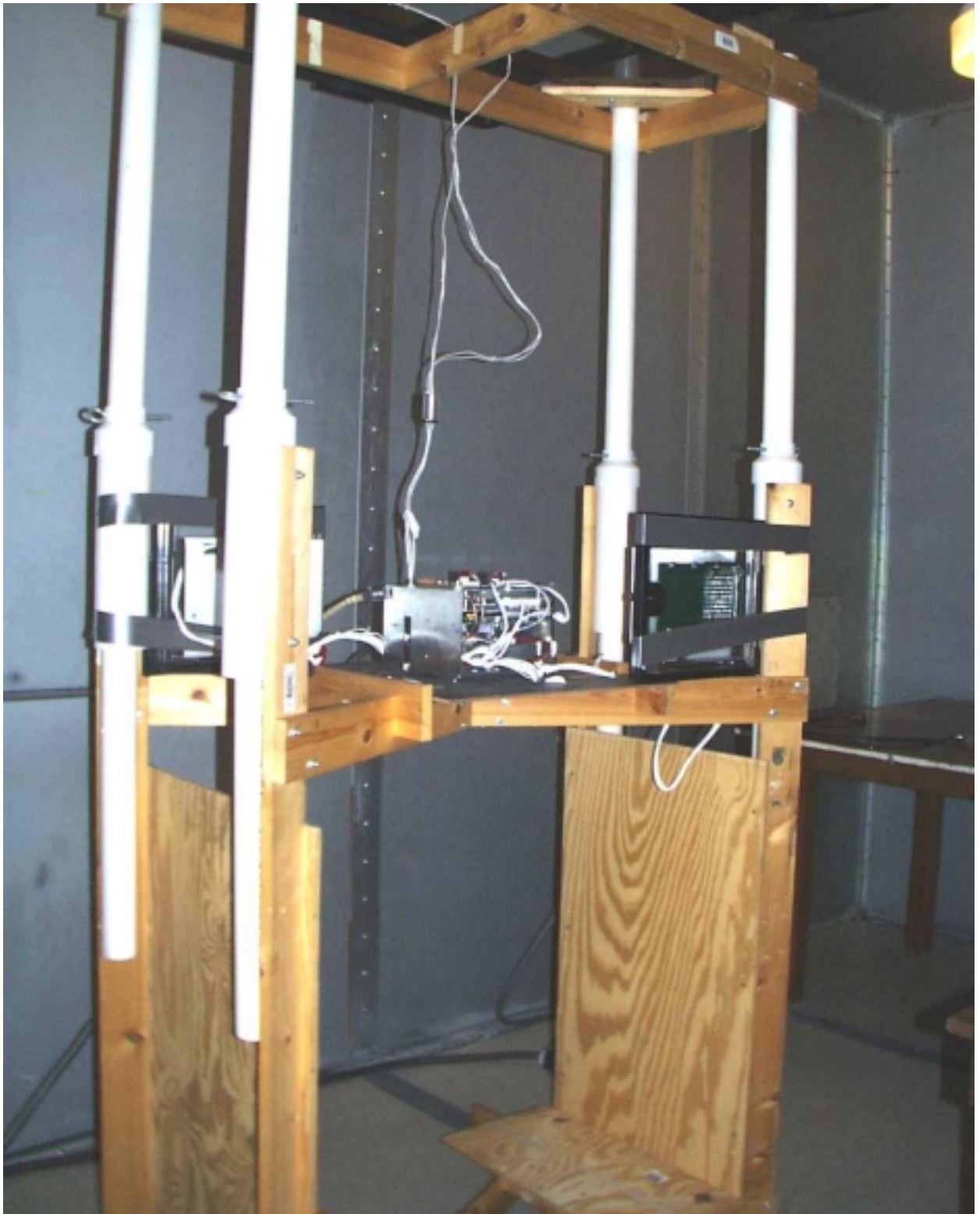
Conducted Emissions Test Setup
