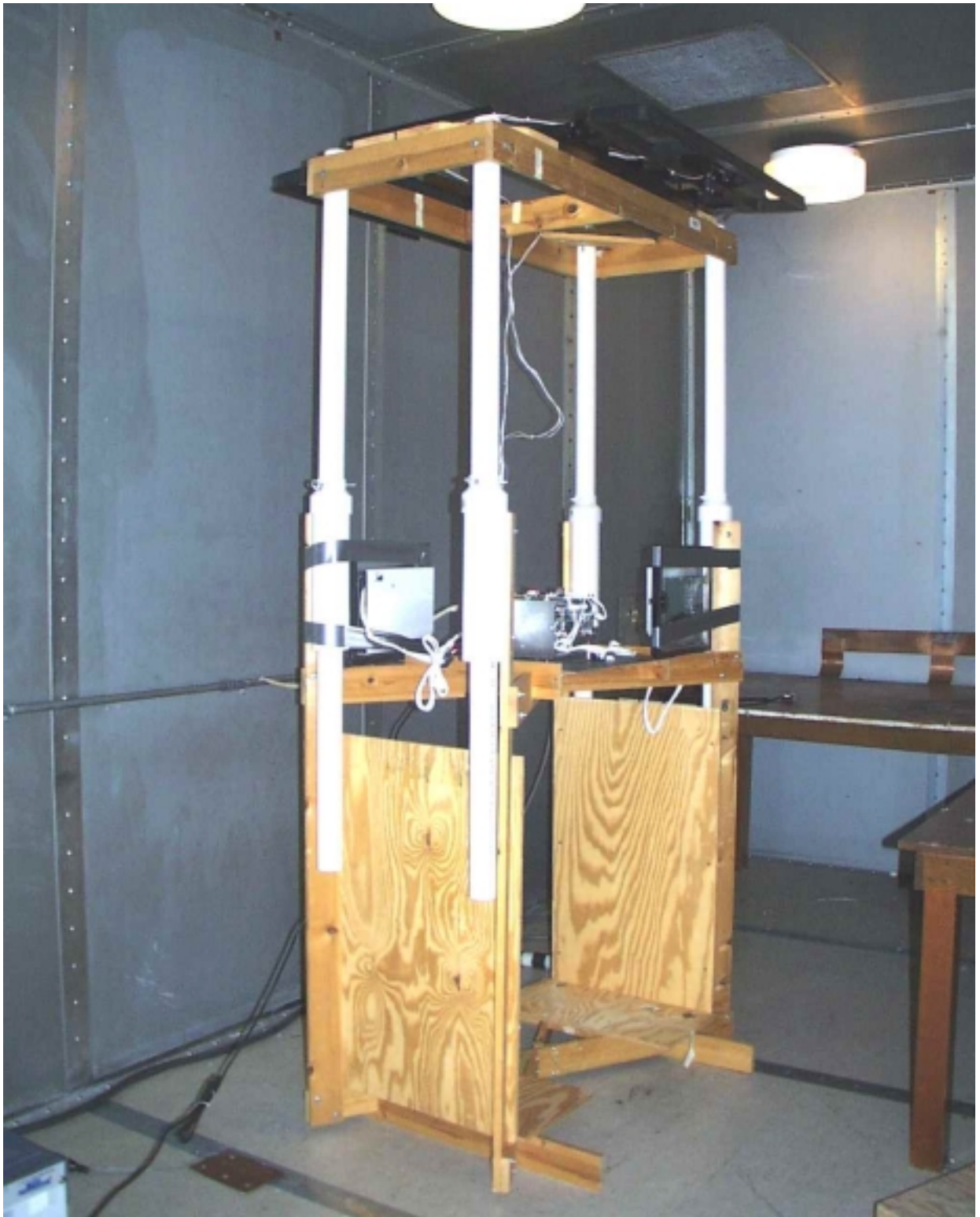
Conducted Emissions Test Setup
