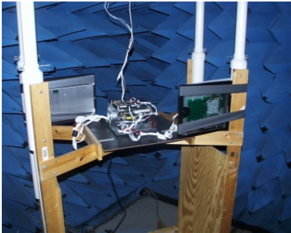
Radiated Emissions Pre-scan (Anechoic) Test Setup
